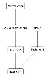
Fig. 3. Native Apollo code gets compiled into Apollo Virtual Machine (AVM) instructions by the compiler front-end. AVM generates standard assembly instructions for regular operations and compiles tensor algebra to t1926 instructions. Respective assemblers target the host CPU and Tachyon 1. This chosen workflow enables tensor algebra to be outsourced to Tachyon 1. Note that the scope of this paper is limited to AVM instruction generation.
