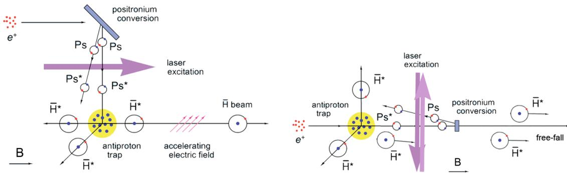
Figure 1 – Left: orthogonal  $\bar{\text{H}}$  production scheme of AEgIS Phase 1: here Rydberg Ps atoms ( $\text{Ps}^*$ ) propagate on average orthogonal to the B field orientation, incurring in the maximal motional Stark effect (see text). Right: collinear  $\bar{\text{H}}$  production scheme of AEgIS Phase 2: here the  $\text{Ps}^*$  atoms propagate on average parallel to the B field, cancelling the motional Stark effect.
