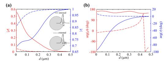
Figure S1. Modulus (a) and argument (b) of the reflection coefficient  $\rho$  (red curves) and transmission coefficient  $\tau$  (blue curves) of the APM at an internal (solid curves) or external nanoscatterer (dashed curves) plotted as a function of the gap *d* between the nanoscatterer and the rim of the microcavity. The insets show the schematics of the two kinds of nanoscatterer and the normalized electric field  $|\mathbf{E}|$  of the fundamental APM.
