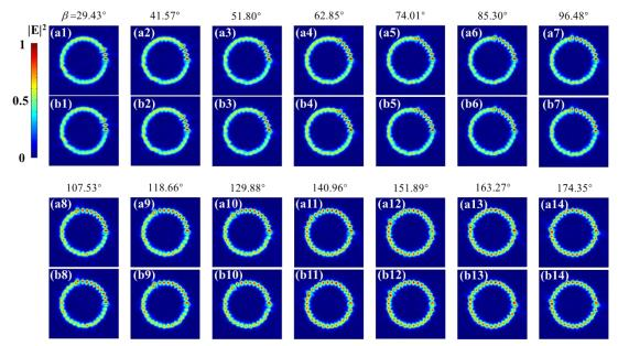
Figure S8. Electric-field intensities  $|\mathbf{E}|^2$  (normalized with a maximum of 1) at the EPs obtained with the FEM shown in Fig. 3 in the main text. The different columns are for different  $\beta$ , and (a1)-(a14) and (b1)-(b14) are for the pair of nearly degenerate resonant modes.
