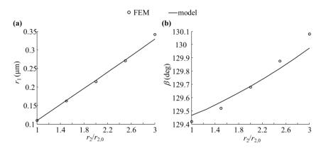
Figure S4. Model predictions (solid curves) and the full-wave FEM results (circles) of  $r_1$  (a) and  $\beta$  (b) at the EPs already shown in Fig. 2.
