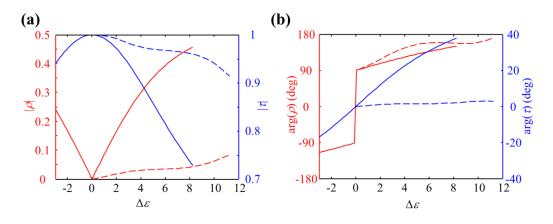
Figure S2. Modulus (a) and argument (b) of the reflection coefficient  $\rho$  (red curves) and transmission coefficient  $\tau$  (blue curves) of the APM at the internal (solid curves) or external nanoscatterer (dashed curves) plotted as a function of  $\Delta \varepsilon$ .
