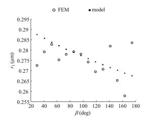
Figure S5. Model predictions (dots) and the FEM results (circles) of  $r_1$  and  $\beta$  at the EPs already shown in Fig. 3.
