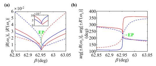
Figure S7. Evolution of the modulus (a) and argument (b) of  $R(\omega_+)$  (blue solid curves),  $-R(\omega_-)$  (red solid curves),  $R'(\omega_+)$  (blue dashed curves) and  $-R'(\omega_-)$  (red dashed curves) as functions of  $\beta$  around the EP [indicated by the green arrows, which is the EP with  $\beta$ =62.85 ° shown in Figs. 3(a) and S6]. The inset in (a) shows a magnification of the region  $\beta \in [62.945^\circ, 62.96^\circ]$  near the EP.
