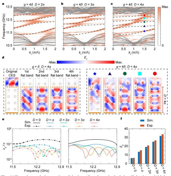
Fig. 4 | Experimental observation of the broadband topological slow light through higher Brillouin zone winding. a-c, Experimentally measured (colour) and numerically calculated
