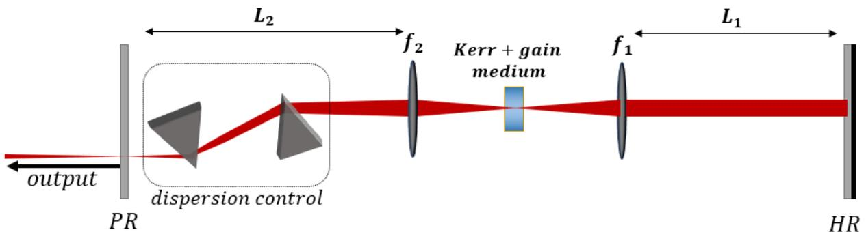
Figure 1. The cavity layout of a standard KLM laser in a linear cavity: The cavity focus is formed by two spherical mirrors / lenses), where the nonlinear Kerr medium (and gain) is placed. Two cavity arms of lengths  $L_1, L_2$  exist around the focus. One of the arms includes components for tuned dispersion control (e.g. a double-prism).
