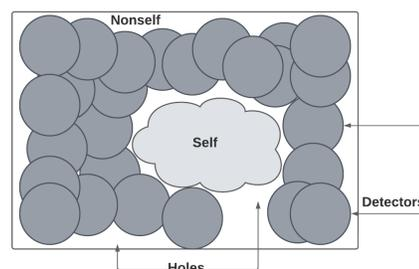
**Figure 2: Negative Selection Algorithm - The candidate detectors, generated randomly, are eliminated if they overlap with self. The ideal set of detectors cover the nonself space and leave minimal holes.**
