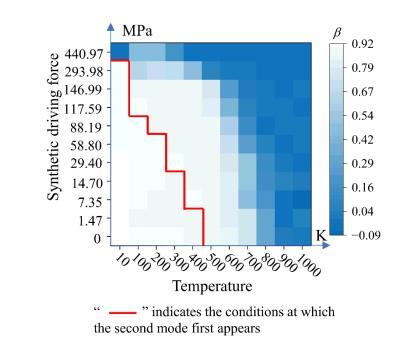
Figure 5 Heatmap of the shear coupling factor in the  $\Sigma$ 15 (2 1 1) Ni GB under varying driving forces and temperatures
