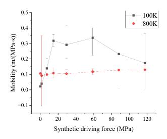
Figure 6 Mobility vs. driving force curves at 100K and 800K for  $\Sigma$ 15 (2 1 1) GB
