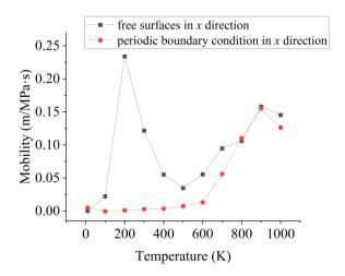
Figure 11 Comparison of the mobility vs. temperature curves for  $\Sigma 15(2\ 1\ 1)$  GB under different boundary conditions
