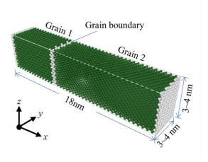
Figure 1 A representative atomistic model of the simulated Ni GBs. Atoms located at perfect FCC sites and non-FCC sites are color-coded in green and white, respectively.
