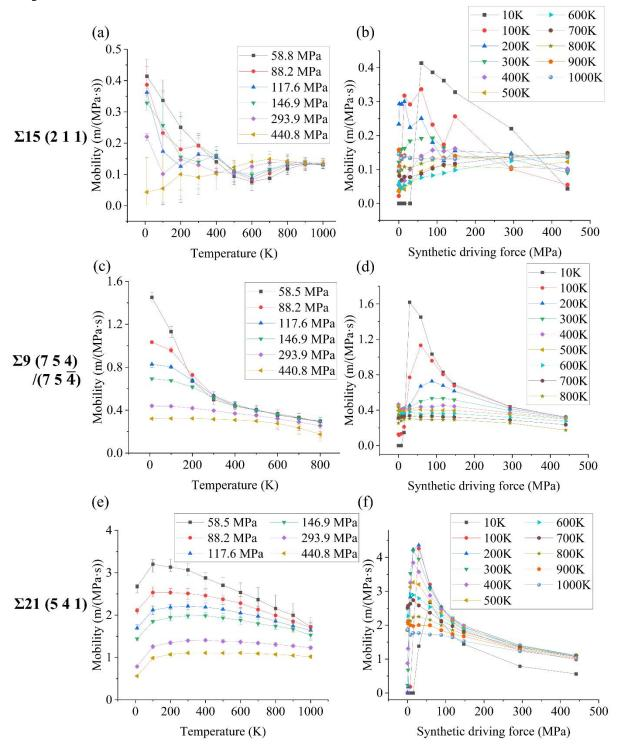
Figure S4 Effect of synthetic driving forces and temperature on GB mobility. (a, c, e) GB mobility vs. temperature curves under various synthetic driving forces ranging from 58.8 to 440.97 MPa. (b, d, f) GB mobility vs. synthetic driving force curves at different temperatures.
