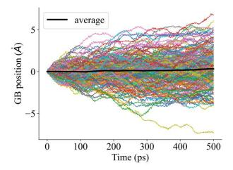
Figure 2 The migration of  $\Sigma$ 15 (2 1 1) GB under the effect of thermal fluctuation at 200K.
