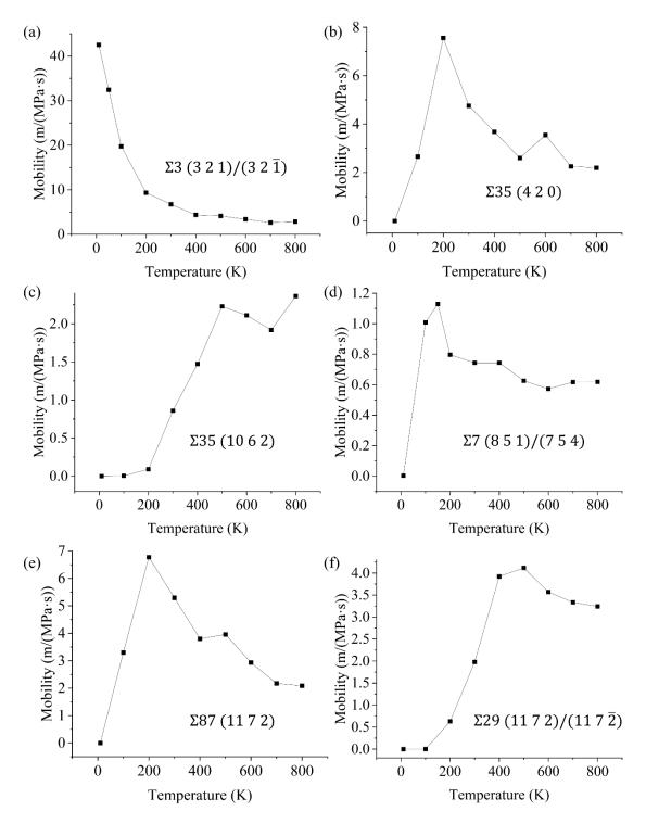
Figure S2 Plots of GB mobility vs. temperature curves of GBs in Table 1 determined by random walk method
