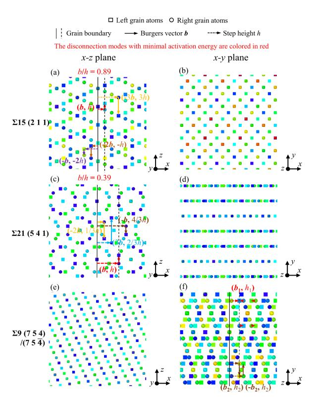
Figure S1 Dichromatic pattern analysis for (a, b)  $\Sigma$ 15 (2 1 1), (c, d)  $\Sigma$ 21 (5 4 1), and (e, f)  $\Sigma$ 9 (7 5 4)/(7 5  $\overline{4}$ ) GBs. The possible disconnection mode associated with the lowest activation energy is marked in red.
