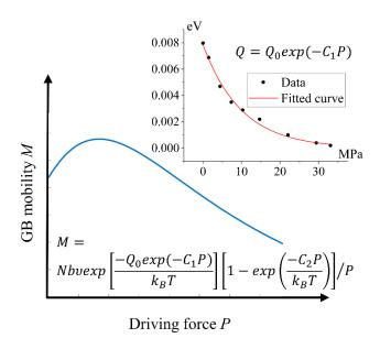
Figure 10 Plot of GB mobility M vs. driving force P based on Eq. 10
