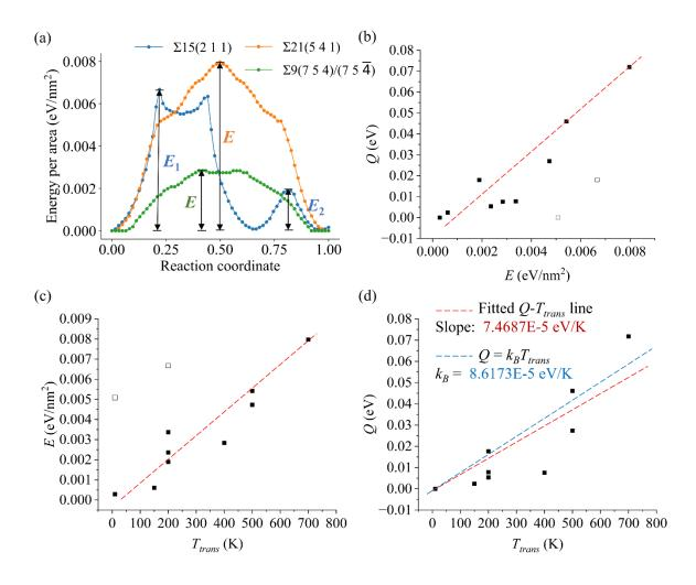
Figure 8 (a) the energy barrier E measured from NEB simulations, and (b) the comparison between E and the apparent activation energy Q. (c, d) Plot of (c) E and (d) Q vs. GB thermal behavior transition temperature  $T_{trans}$  ( $\Box$  indicates the second energy barrier E for GBs with two distinct energy barriers)
