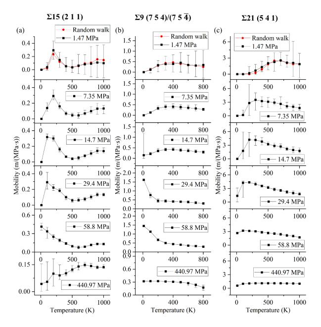
Figure 4 The effect of synthetic driving force on GB mobility for (a)  $\Sigma 15$  (2 1 1), (b)  $\Sigma 9$  (7 5 4)/(7 5  $\overline{4}$ ), and (c)  $\Sigma 21$  (5 4 1) GBs in Ni.
