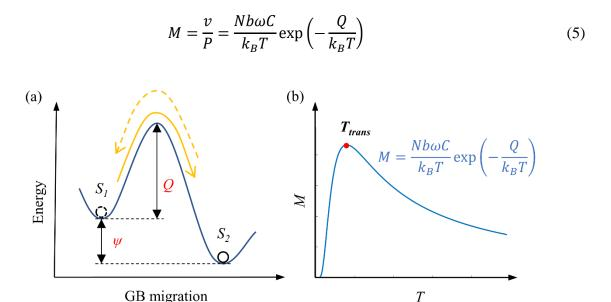
Figure 7 (a) Illustration of the classical thermal-activation model [24] and (b) Plot of the mobility vs. temperature curve based on Eq. 5
