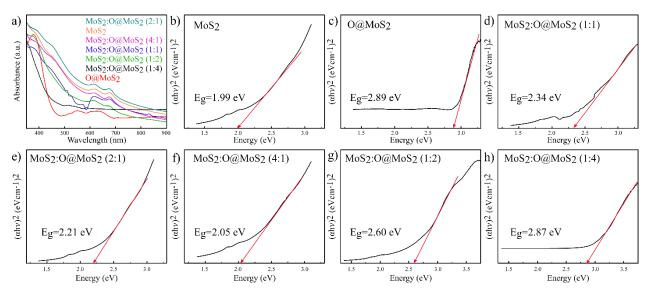
**Fig. 4.** (a) UV-Visible spectra of all introduced suspensions. Tauc plots of (b)  $MoS_2$ , (c) O@MoS\_2, and  $MoS_2$ :O@MoS\_2 with different mass ratios of (d) 1:1, (e) 2:1, (f) 4:1, (g) 1:2, and (h) 1:4.
