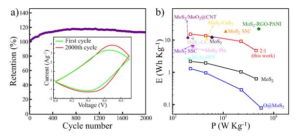
**Fig. 6. (a)** Cyclic stability of  $MoS_2:O@MoS_2$  (2:1) electrode after 2000 cycles at 200 mVs<sup>-1</sup> scan rate. **Inset**: The first and last cycles after 2000 continuous charge and discharge cycles. (b) Ragone plot of the  $MoS_2$ ,  $O@MoS_2$  and  $MoS_2:O@MoS_2$  (2:1) electrodes.
