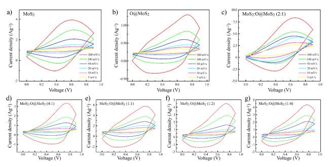
**Fig. 5.** CV curves of the (**a**) MoS<sub>2</sub>, (**b**) O@MoS<sub>2</sub>, and MoS<sub>2</sub>:O@MoS<sub>2</sub> with different mass ratio of (**c**) 2:1, (**d**) 4:1, (**e**) 1:1, (**f**) 1:2, and (**g**) 1:4 at scan rates of 5 mVs<sup>-1</sup> to 200 mVs<sup>-1</sup>.
