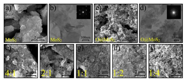
**Fig. 3.** SEM and TEM characterizations of the prepared samples. (a) SEM, and (b) TEM images of the pristine  $MoS_2$  flakes. (c) SEM, and (d) TEM images of the  $O@MoS_2$  flakes. SEM image of (e) 4:1, (f) 2:1, (g) 1:1, (h) 1:2, and (i) 1:4 composites.
