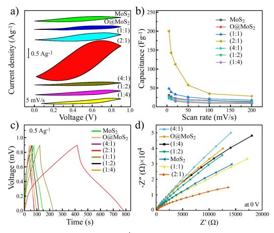
**Fig. 5.** (a) CV curves of electrodes at a 5 mVs<sup>-1</sup> scan rate, (b) Gravimetric capacitance of electrodes as a function of scan rate, (c) GCD curves at current density of 0.5 Ag<sup>-1</sup>, and (d) Nyquist diagrams of electrodes.
