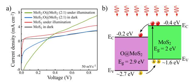
Fig. 7. (a) Linear sweep voltammetry measurements of the  $MoS_2:O@MoS_2$  (2:1) and  $MoS_2$  electrodes under visible light irradiation and in dark. (b) Depiction of charge separation process in the  $MoS_2:O@MoS_2$  (2:1) hybrid.
