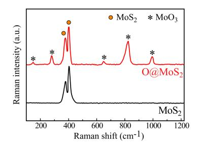
Fig 2. Raman spectra of the pristine and thermally treated MoS<sub>2</sub> flakes at 500 °C for 60 min.
