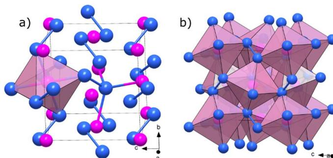
Figure 4: Crystal structure of  $\text{PN}_2$  at 134 GPa, where the blue and pink spheres represent nitrogen and phosphorus atoms, respectively. a) Unit cell with a single  $\text{PN}_6$  octahedra and the four bonds of the  $\text{N}^{[4]}$  center drawn. b) Unit cell with all  $\text{PN}_6$  octahedra shown.
