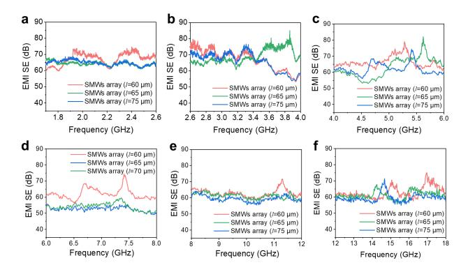
**Fig. 4 EMI SE comparison of SMW arrays** (*d*=1 mm). EMI SE of SMW arrays with varying structural parameters at different frequency band. **a** 1.7–2.6 GHz. **b** 2.6–4 GHz. **c** 4–6 GHz. **d** 6–8 GHz. **e** 8–12 GHz. **f** 12–18 GHz
