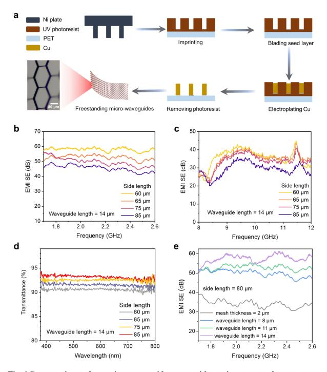
Fig. 6 Comparative study on micro-waveguides array with varying structural parameters. a Fabrication process of metallic hexagonal micro-waveguides using additive manufacturing method. The freestanding apertured micro-structures with high aspect ratios obtained by peeling off from the PET substrate. b EMI shielding performance of separate micro-waveguide array ( $t = 14 \mu m$ ) with varying side lengths in the frequency range of 1.7–2.6 GHz. c 8–12 GHz.
