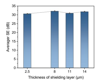
Fig. S5 Average shielding performance of thin metal mesh (2.5  $\mu$ m in thickness) and freestanding micro-waveguide layers with varying waveguide lengths (8  $\mu$ m, 11  $\mu$ m, 14  $\mu$ m) in X-band. The side lengths of apertures are 80  $\mu$ m.
