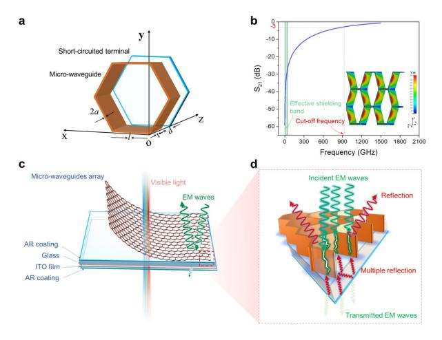
**Fig. 1 Design concept of SMW array. a** The unit structure of shorted micro-waveguides array. **b** The simulated transmission characteristic of micro-waveguide, and the inset is the electric field distribution of EM waves at 10 GHz. **c** Schematic diagram structure of shorted micro-waveguides array for achieving high optical transparency and superior electromagnetic shielding. **d** Principle diagram of EMI shielding mechanism of shorted micro-waveguides array
