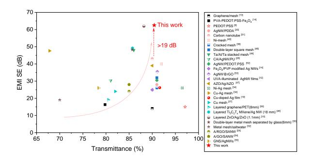
Fig. 5 Comparison of average EMI SE and optical transmittance for our transparent EMI shielding material with previously reported results. Our work can outperform the prior transparent EMI shielding materials at the corresponding transparency
