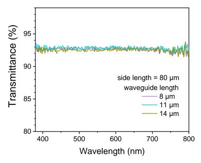
Fig. S4 Optical transmittance of freestanding micro-waveguides (side length =  $80 \mu m$ ) with different waveguide lengths. Since there is no change in light transmission aperture, they exhibit almost identical light transmission.
