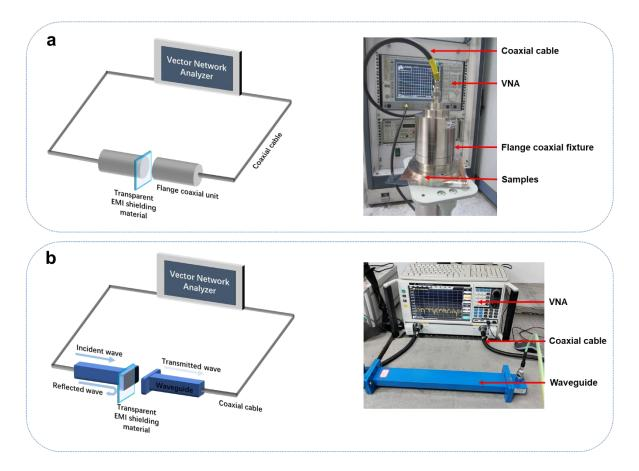
**Fig. S6 EMI SE measurement set-up. a** Schematic diagram and the experimental setup of the Flanged coaxial EMI SE measurement fixture used in the frequency range from 0.03 GHz to 1.5 GHz. **b** Waveguide measurement system employed in the frequency range from 1.7 GHz to 18 GHz. We used six sets of waveguides operated in various frequency bands (1.7–2.6 GHz, 2.6–4 GHz, 4–6 GHz, 6–8 GHz, 8–12 GHz, and 12–18 GHz) to obtain data over broadband frequencies.
