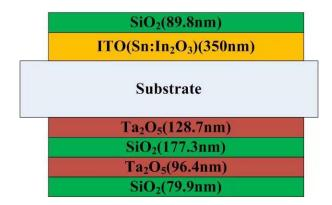
**Fig. S1 Anti-reflection design for the thin glass with ITO.** A  $SiO_2$  film of 89.8 nm was deposited on the surface of ITO film.  $Ta_2O_5$  and  $SiO_2$  films are deposited alternately on the other side of the substate. The thicknesses of the films are 128.7 nm, 177.3 nm, 96.4 nm, and 79.9 nm, respectively.
