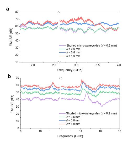
**Fig. 3 Effect of insulation distance** (*d*) **on EMI SE.** EMI shielding performance of SMW array with varying insulation distance (*d*) in varying frequency range. **a** 1.7–4 GHz. **b** 8–18 GHz
