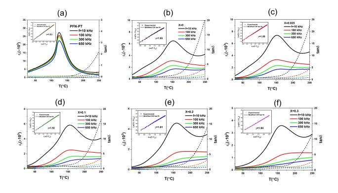
Figure 3: Temperature dependence of relative permittivity ( $\epsilon'$ ) (solid lines) and the corresponding dielectric loss tangent (tan $\delta$ ) (dashed lines) in frequency range of 10 to 650 kHz for (PFN-PT)-(CF<sub>2-x</sub>Z<sub>x</sub>O) composites samples with (a) x=0, (b) x=0.025, (c) x=0.1, (d) x=0.2, (e) x=0.3, as well as pure PFN-PT (f). Insets show fits of data above transition temperature to modified Curie-Weiss law.
