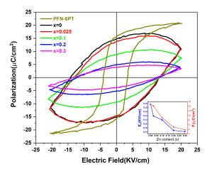
Figure 4: Room temperature polarization-electric field (P-E) loops of (PFN-PT)-(CF<sub>2-x</sub> $Z_x$ O) composites samples, as well as pure PFN-PT, measured at a frequency of 50 Hz. Inset shows the coercive field (Ec) and remnant polarization (Pr) as a function of Zn content.
