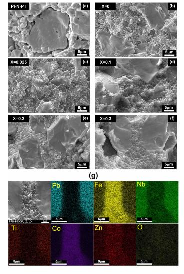
Figure 2: (a-f) FE-SEM images of the sintered pellets of the pure PFN-PT as well as (PFN-PT)-( $CF_{2-x}Z_xO$ ) composites samples (with x=0, x=0.025, x=0.1, x=0.2, x=0.3). (g) EDS mapping images for the sample PFN-PT- $CoFe_{1,7}Zn_{0.3}O_4$ .
