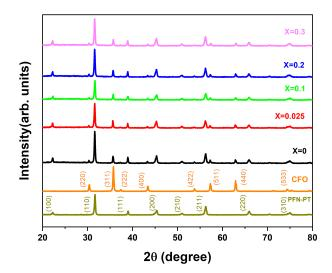
Figure 1: XRD patterns of (PFN-PT)-( $CF_{2-x}Z_xO$ ) composites (x=0, x=0.025, x=0.1, x=0.2, x=0.3) as well as pure PFN-PT and CFO.
