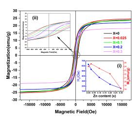
Figure 5: Room temperature magnetization loops of (PFN-PT)-( $CF_{2-x}Z_xO$ ) composites. Inset (i) shows the coercive field ( $H_c$ ) and saturation magnetization ( $M_s$ ) as a function of Zn content. Inset (ii) shows a zoomed view of the m-h loop in the vicinity of the center.
