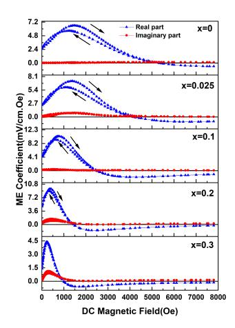
Figure 6: Real and imaginary part of transverse ME voltage coefficient  $(\alpha_{31}^*)$  as a function of DC magnetic field for (PFN-PT)-(CF<sub>2-x</sub>Z<sub>x</sub>O) composites (x=0, x=0.025, x=0.1, x=0.2, x=0.3), h<sub>ac</sub>=0.77 Oe, and f=978 Hz.
