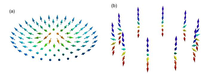
FIG. 1. Ring spin configuration (12) at the initial time t = 0 for the magnetic length  $\ell_0 = 0.7 \text{ nm}$ , parameter  $\tilde{r}_0 = 50 \ell_0$  and the thickness of the spin texture  $d \approx 5 \text{ nm}$ . (a) Ring spin texture. (b) Magnetization configuration and turn of the polar angle  $\theta$  by  $-\pi$  from  $\theta = \pi$  at  $z \approx -2.5 \text{ nm}$  to  $\theta = 0$  at  $z \approx 2.5 \text{ nm}$  for a fixed radius between inner and outer ones.
