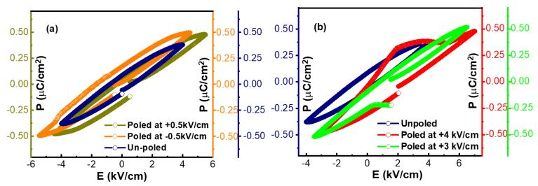
Figure 4(a): P-E hysteresis loop of un-poled and poled sample at  $\pm 0.5$  kV/cm electric field, (b) Un-poled and poled sample at +3 and +4 kV/cm electric field at 100 Hz frequency of heat treated Ti<sub>3</sub>C<sub>2</sub>T<sub>x</sub> MXene film measured at room temperature.
