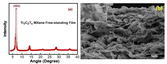
Figure 2: (a) XRD pattern of  $Ti_3C_2T_x$  MXene Free-standing Film, (b) SEM image of  $Ti_3C_2T_x$  MXene Free-standing film.
