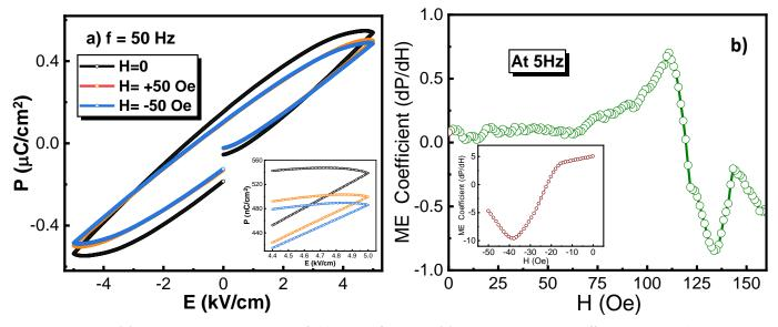
Figure 5: (a) The P-E loop in static magnetic field at 50 Hz frequency, (b) The magnetoelectric coefficient versus applied DC magnetic field at 5Hz frequency of heat treated Ti<sub>3</sub>C<sub>2</sub>T<sub>x</sub> MXene film measured at room temperature.
