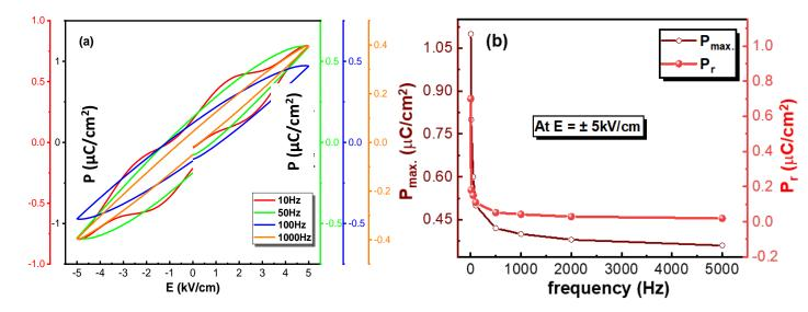
Figure 3: (a) Ferroelectric hysteresis loops at different frequency ranges, (b)  $P_r$ ,  $P_{max}$  versus frequency ranges at  $\pm 5$  kV/cm of heat treated  $Ti_3C_2T_x$  MXene film measured at room temperature.
