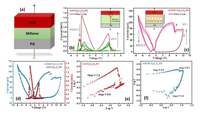
Figure 6: (a) schematic representation of trilayer memory device. (b) Resistive switching behavior of rGO/  $Ti_3C_2T_x$  /Pd and (c)  $rGO/HT-Ti_3C_2T_x/Pd$ , (d) first cycle of both rGO/ $Ti_3C_2T_x/Pd$  and rGO/HT- $Ti_3C_2T_x/Pd$  memory devices, (e) double logarithmic graph of  $rGO/Ti_3C_2T_x/Pd$  as well as (f) rGO/HT- $Ti_3C_2T_x/Pd$  memory device.
