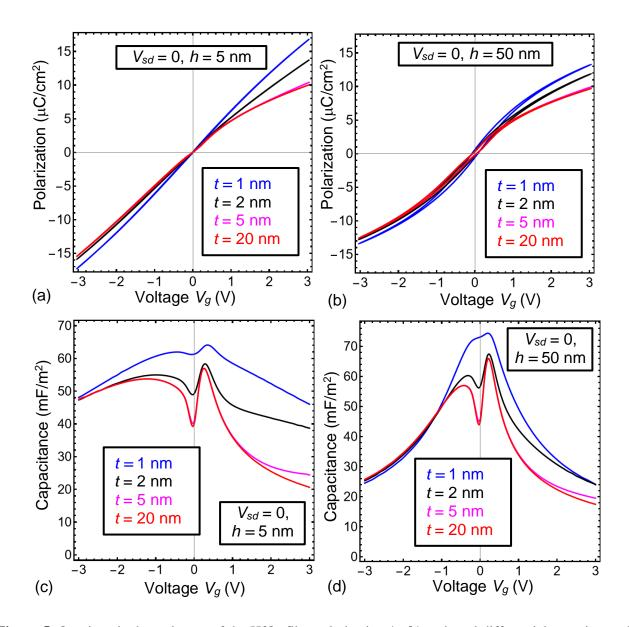
Figure 5. Quasi-static dependences of the HfO<sub>2</sub> film polarization (**a**, **b**) and total differential capacitance (**c**, **d**) on the reduced gate voltage  $V_g$  calculated for different channel widths t=1, 2, 5 and 20 nm (blue, black, magenta and red curves, respectively). The HfO<sub>2</sub> film thickness h=5 nm in the plots (**a**, **c**) and h=50 nm in the plots (**b**, **d**).
