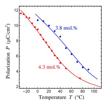
**Figure B1**. Temperature dependence of the polarization for the different degree of Si doping, namely 3.8 and 4.3 molar % (blue and red curves/symbols respectively). Points represent experimental results from [26], while curves represent the fitting with Eq.(A1). LGD parameters are summarized in Table I.
