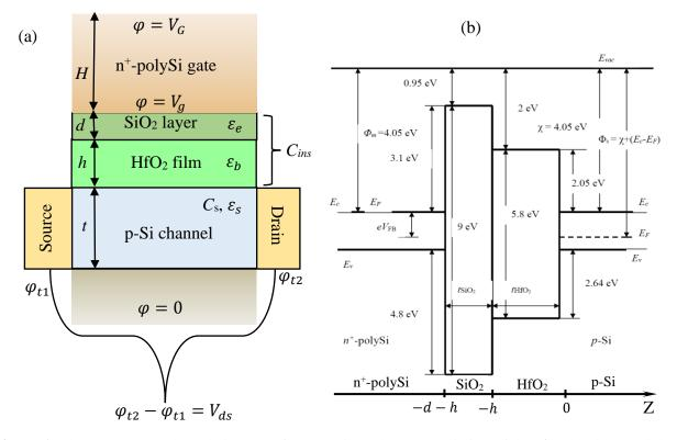
**Figure 1.** The geometry and band diagram of the considered FET, consisting of the  $n^+$  poly-Si gate, dielectric SiO<sub>2</sub> layer, ferroelectric HfO<sub>2</sub> film, and the p-type Si channel.
