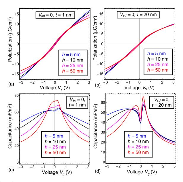
**Figure 4**. Quasi-static dependences of the HfO<sub>2</sub> film polarization (**a**, **b**) and total differential capacitance (**c**, **d**) on the reduced gate voltage  $V_g$  calculated for different thickness of HfO<sub>2</sub> film h=5, 10, 25 and 50 nm (blue, black, magenta and red curves, respectively). The channel width t=1 nm in the plots (**a**, **c**) and t=20 nm in the plots (**b**, **d**).
