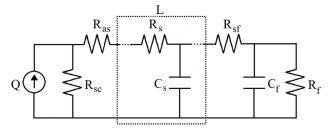
Fig. 3. Equivalent thermo-physical circuit model of the sample in contact with the copper holder, where Q is the input radiation power,  $C_f$  is the lumped heat capacitance of the film, Cs and Rs are the heat capacity and the thermal resistivity of the substrate material, respectively,  $R_{sf}$ ,  $R_{as}$  and  $R_{sc}$  are the thermal boundary resistance values at the substrate/YBCO film, absorber/substrate and the substrate/coper holder interfaces, respectively.
