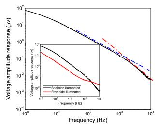
Fig. 5. The voltage amplitude response of the fabricated free-membrane bolometer. Inset: the voltage response of the fabricated bolometer in black: backside illuminated, and red: front-side illuminated case.
