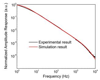
Fig. 6. The simulated and measured voltage amplitude response of the fabricated free-membrane bolometer.
