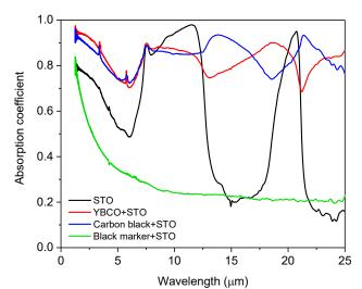
Fig. 4. The absorption coefficient of STO substrate, and superconducting YBCO thin film, carbon black, and black marker on STO substrate.
