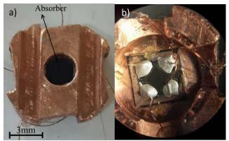
Fig. 2. a) The copper sample holder for free-standing substrate (The absorber layer on the backside of the device is seen at the middle of the sample holder), b) the fabricated bolometer mounted on the sample holder (electrical contact was implemented using silver paste and copper wires, and the absorber was applied on the backside of the device).
