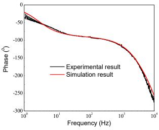
Fig. 7. The simulated and measured voltage phase response of the fabricated free-membrane bolometer.
