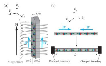
Figure 2: Magnetization of the beam specimen. (a) The beam was magnetized while folded at the mid-span, s = L/2, inside a pulse magnetizer, which generates a strong axial magnetic field, **H**. (b) After unfolding, the magnetized specimen exhibited the antiparallel residual magnetic flux density of **B**<sup>r</sup> described in Eq. (1). Two non-magnetic cubic blocks attached to the extremities ensured clamped boundary conditions.
