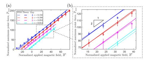
Figure 8: Critical indentation load for snap-transition under magnetic actuation. (a) Normalized maximum indentation force,  $\overline{P}_{max}$ , versus the prescribed applied magnetic field,  $\overline{B}^a$ , at different end-to-end shortenings ( $\epsilon = \{0.158, 0.108, 0.053, 0.014\}$ ): experiments (data points), theoretical predictions from Eq. (13) (solid lines), and FEM (dotted lines). (b) Zoomed view of (a) with a depicted slope of 2, consistently with Eq. (20).
