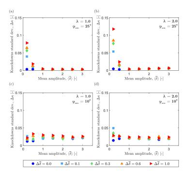
Figure 9: Standard deviation of the resultant knockdown factors,  $\Delta \kappa$ , versus the mean defect amplitude,  $\langle \bar{\delta} \rangle$ . (a, b)  $\varphi_{\min} = 25^{\circ}$  (non-interacting defects) and widths  $\lambda = 1$  and  $\lambda = 2$ , respectively. (c, d)  $\varphi = 10^{\circ}$  (interacting defects) and widths  $\lambda = 1$  and  $\lambda = 2$ , respectively. The various datasets correspond to different values of  $\Delta \bar{\delta}$  (see legend).
