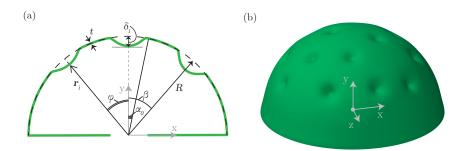
Figure 1: Problem Definition. (a) A two-dimensional schematic of an elastic hemispherical shell with three dimple defects. (b) A three-dimensional representation of a shell with multiple dimple imperfections,  $w_i$  (Eq. 3), whose amplitudes,  $\bar{\delta}_i$ , follow a lognormal distribution (Eq. 7).
