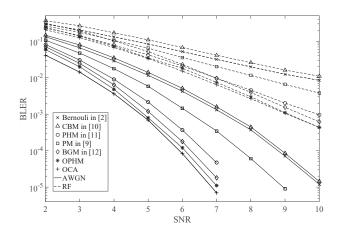
Figure 2. BLER performance comparison between the proposed spreading matrices and the counterparts in [2], [9]–[12], where  $C \in \{+1, -1\}^{15 \times 24}$ .
