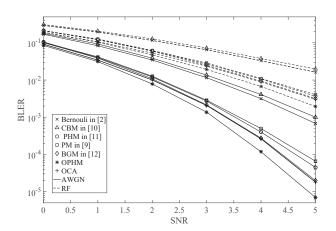
Figure 3. BLER performance comparison between the proposed spreading matrices and the counterparts in [2], [9]–[12], where  $\mathbf{C} \in \{+1, -1\}^{20 \times 24}$ .
