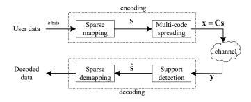
Figure 1. The block diagram of SVC.
