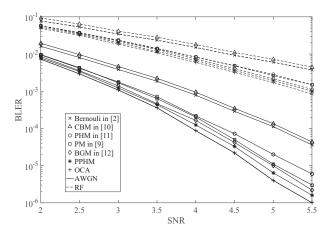
Figure 4. BLER performance comparison between the proposed spreading matrices and the counterparts in [2], [9]–[12], where  $\mathbf{C} \in \{+1, -1\}^{25 \times 65}$ .
