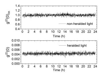
FIG 3.  $g^{(2)}(0)$  and  $g^{(2)}(0)_{nh}$  measured through 24 hours. Black line represents value of  $g^{(2)}(0)$  and  $g^{(2)}(0)_{nh}$  for measurements collected every minute. Note the different vertical scale on the two graphs.
