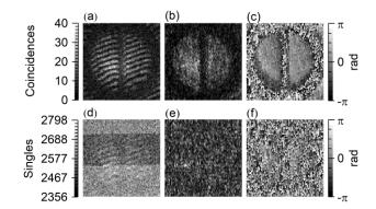
FIG 4. Upper row: hologram recorded with single-photon states (a); corresponding amplitude (b); and phase (corrected) reconstruction (c). Lower row: hologram recorded with non-heralded light (d); corresponding amplitude (e); and phase (corrected) reconstruction (f). Coincidence noise and noise of the imaging detector is not subtracted from the shown counts.
