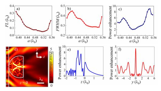
Fig. 3. Numerical results of the (a) *FL*, (b) *FWHM* and (c) power enhancement as a function of *a* for a truncated 2D dielectric cylinder with  $R = 1.55\lambda_0$ . (d) Power enhancement on the *yz*-plane for  $R = 1.55\lambda_0$  and  $a \approx 0.52\lambda_0$ . Power enhancement along (e) the *z*-axis at y = 0 and (f) *y*-axis at the *FL*, extracted from panel (d).
