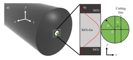
Fig. 1. (a) Schematic representation of the optical fiber with the mesoscale dielectric particle placed at its end and immersed in air. (b) Side view of (a). The red line represents the power distribution of the fundamental mode inside the fiber. The design parameters for the truncated mesoscale dielectric structure are also shown in (b).
