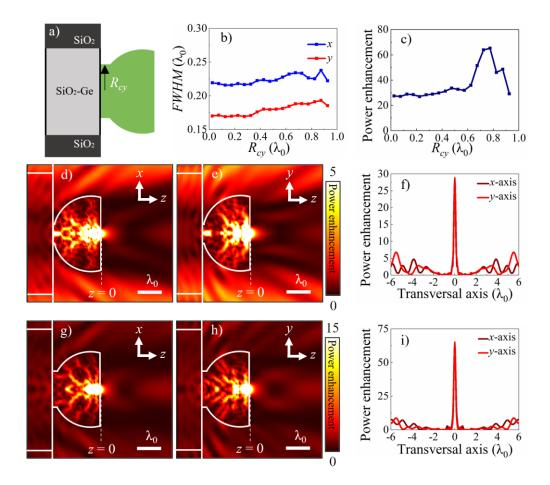
Fig. 6. (a) Shows the schematic of Fig. 4d when the cylinder is added to the back side of the truncated spherical dielectric with radius  $R_{cy}$ . (b,c) Presents the *FWHM*<sub>xy</sub> and the power enhancement with different cylinder radius  $R_{cy}$ . (d-f) and (g-i) Show the power enhancement on the *xz*-plane at y = 0, *yz*-plane at x = 0, and transverse *x*- and *y*-axes at z = 0 for  $R_{cy} = 0.325\lambda_0$  and  $R_{cy} = 0.775\lambda_0$ , respectively.
