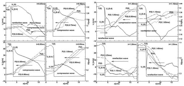
Fig. 13(a, b). Sequences of pressure and velocity distribution along the center line, and the flow velocity profiles  $U_+(x, y = 0)$  and  $U_+(x, y = 0.4)$ ; L=18cm.
