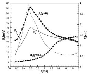
Fig. 14. Calculated time evolution of combustion wave velocity  $S_f$ , the flame surface area  $F_f$  (dashed-dotted) and local velocities of the flame front at y=0 and near the sidewall at y=0.4 cm for the half-open tube.
