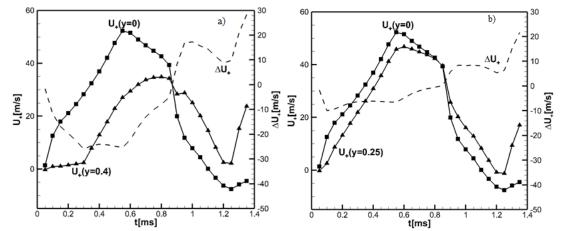
Fig. 11(a, b). Velocities of the flow at 1 mm ahead of the flame front at y=0, 0.4, 0.25 cm and the difference  $\Delta U_+$  between  $U_+(y=0.4), U_+(y=0.25)$  and  $U_+(y=0)$ ; L=18 cm.
