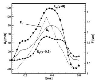
Fig. 19. Time evolution of the flame surface area  $F_f$  (dashed-dotted), local velocities of the flame front at y=0 and at y=0.3 cm, and combustion wave velocity  $S_f$ , for the tube with both closed ends, L/D=6.
