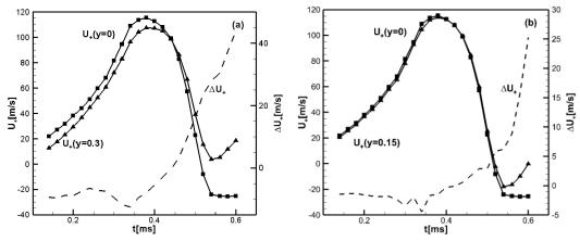
**Fig. 20** (a, b). The flow velocities at 1mm ahead of the flame front at the cross section (x, y, z = 0), at y = 0, y = 0.15cm, and y = 0.3cm; and  $\Delta U_+ = U_+(y = 0.15$ cm)  $-U_+(y = 0)$  and  $\Delta U_+ = U_+(y = 0.3$ cm)  $-U_+(y = 0)$ .
