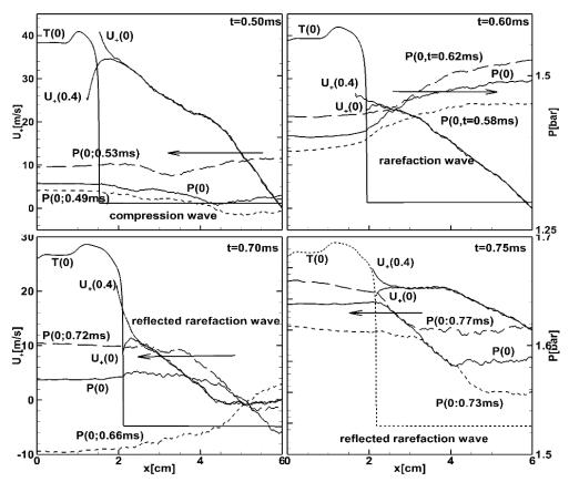
Fig. 7(a) Sequences of pressure and velocity distribution along the center line, and the flow velocity profiles  $U_+(x, y=0)$  and  $U_+(x, y=0.4)$  before the flame front flattering.
