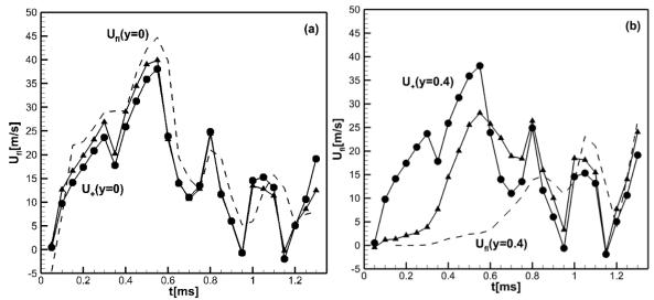
**Fig. 3** (a, b). a) Flame front velocity at y = 0 (dashed line) and flow velocity at  $1 \text{mm}(\blacktriangle)$  and  $3 \text{ mm}(\bullet)$  ahead of the flame front. b) Flame front velocity at y = 0.4 cm (dashed line) and flow velocity  $1 \text{mm}(\bigstar)$  and  $3 \text{ mm}(\bullet)$  ahead of the flame front.
