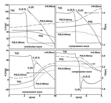
Fig. 23. Sequences of pressure profiles along the center line and the flow velocities ahead of the flame at y=0 and y=0.3 cm; 3D tube L=6 cm, cross section  $1 \times 1$  cm<sup>2</sup>.
