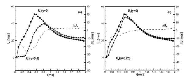
**Fig. 16(a, b)**. Velocities of the flow at 1 mm ahead of the flame front at y = 0, 0.25 0.4cm and the difference  $\Delta U_+$  between  $U_+(y=0.4cm), U_+(y=0.25cm)$  and  $U_+(y=0)$ ; half open tube.
