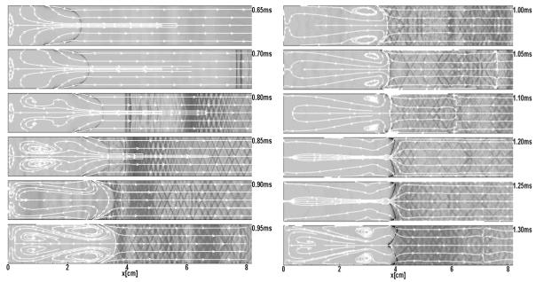
Fig. 9 Schlieren images and stream lines for the premixed hydrogen/air flame propagating in the tube with both closed ends, aspect ratio L/D=18.
