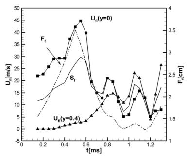
Fig. 2. Time evolution of combustion wave velocity  $S_f$ , local velocities of the flame front at y=0 and at y=0.4 cm and the flame surface area  $F_f$  (dashed-dotted), tube L/D=6.
