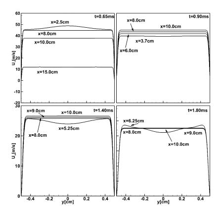
Fig. 17. Axial velocity profiles in the flow ahead of the flame in various cross sections of the half-open tube.
