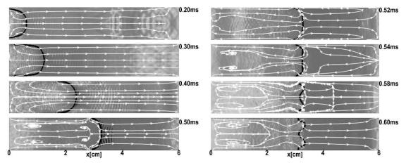
Fig. 21 (a, b). Schlieren images and stream lines; premixed hydrogen/air flame propagating in the 3D tube with both closed ends L = 6 cm, cross section  $1 \times 1$  cm<sup>2</sup>; shown is cross section (x, y, z = 0).
