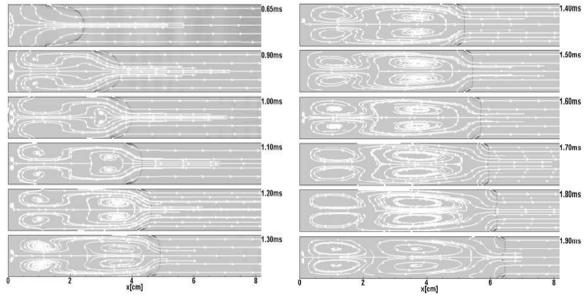
Fig. 15(a, b). Sequences of computed Schlieren images and the stream lines for the premixed hydrogen–air flame propagating to the right open end.
