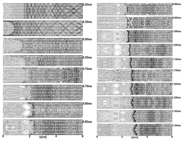
Fig. 1(a,b-c,d). Time sequence of computed Schlieren images and streamlines for the flame propagating in the tube L/D=6 with both ends closed.
