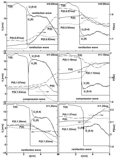
Fig. 7(b) Sequences of pressure and velocity distribution along the center line, and the flow velocity profiles  $U_+(x, y=0)$  and  $U_+(x, y=0.4)$  during the tulip flame formation.
