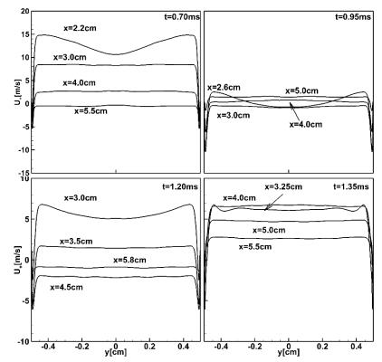
Fig. 5. Velocity profiles in the flow ahead of the flame in different cross sections of the tube.
