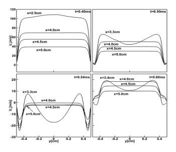
Fig. 22. 3D LES simulations: velocity profiles in the flow ahead of the flame in different cross sections of the tube.
