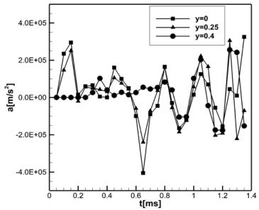
Fig. 6. Calculated accelerations at various points at the flame front during the tulip flame formation.
