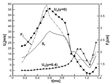
Fig. 10. Evolution of combustion wave velocity  $S_f$ , the flame surface area  $F_f$ , and local velocities of the flame front at y=0 and at y=0.4 cm for the tube L=18 cm.
