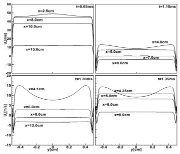
Fig. 12. Axial velocity profiles in the flow ahead of the flame front at selected times of the tulip flame formation. Figure 13(a, b) shows the sequences of pressure profiles P(x, y = 0) and the flow velocity
