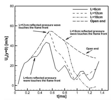
Fig. 8. The velocity of the flame tip along the center line y=0, computed for tubes L/D=6,12,18 and the half-open tube.
