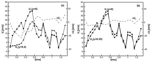
Fig. 4 (a, b). Velocities of the flow at 1 mm ahead of the flame front at y=0; 0.4; 0.25cm, and the difference  $\Delta U_+$  between  $U_+(y=0.4)$ ,  $U_+(y=0.25)$  and  $U_+(y=0)$ .
