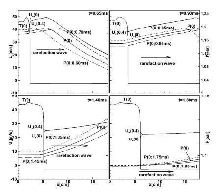
Fig. 18. Pressure and the flow velocity profiles ahead of the flame during the development of the tulip flame for half open tube.
