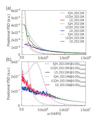
Fig. 4. (a) Positional PSD at 253.15 and 333.15 K for the perforated Au plate of 0.17  $\mu$ m with a critical perforation lattice constant. The prime symbol denotes that the spectrum at 253.15 K is calculated with the same viscosity at 333.15 K (0.58 cP). (b) Positional PSD of the same perforated Au plate under 1/20-fold  $\gamma_c$ . The pink and green lines are the smoothed LD spectra.
