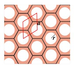
Fig. S2. Illustration of square Au plate perforated with hexagonal lattice of circular hole.
