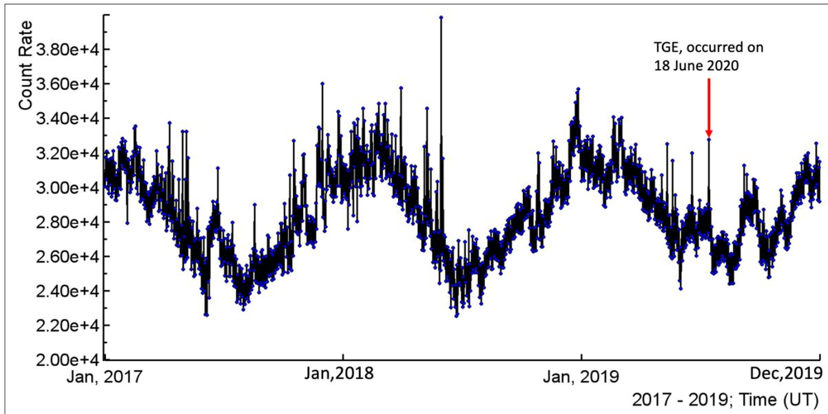
**Figure 2.** 1-minute time series of count rates of 3 cm thick scintillator of the STAND3 detector, energy threshold 4 MeV used for TGE identification (covering 3 years' time span). By the arrow, we show one of the registered TGEs, its zoomed version will appear in the next picture.
