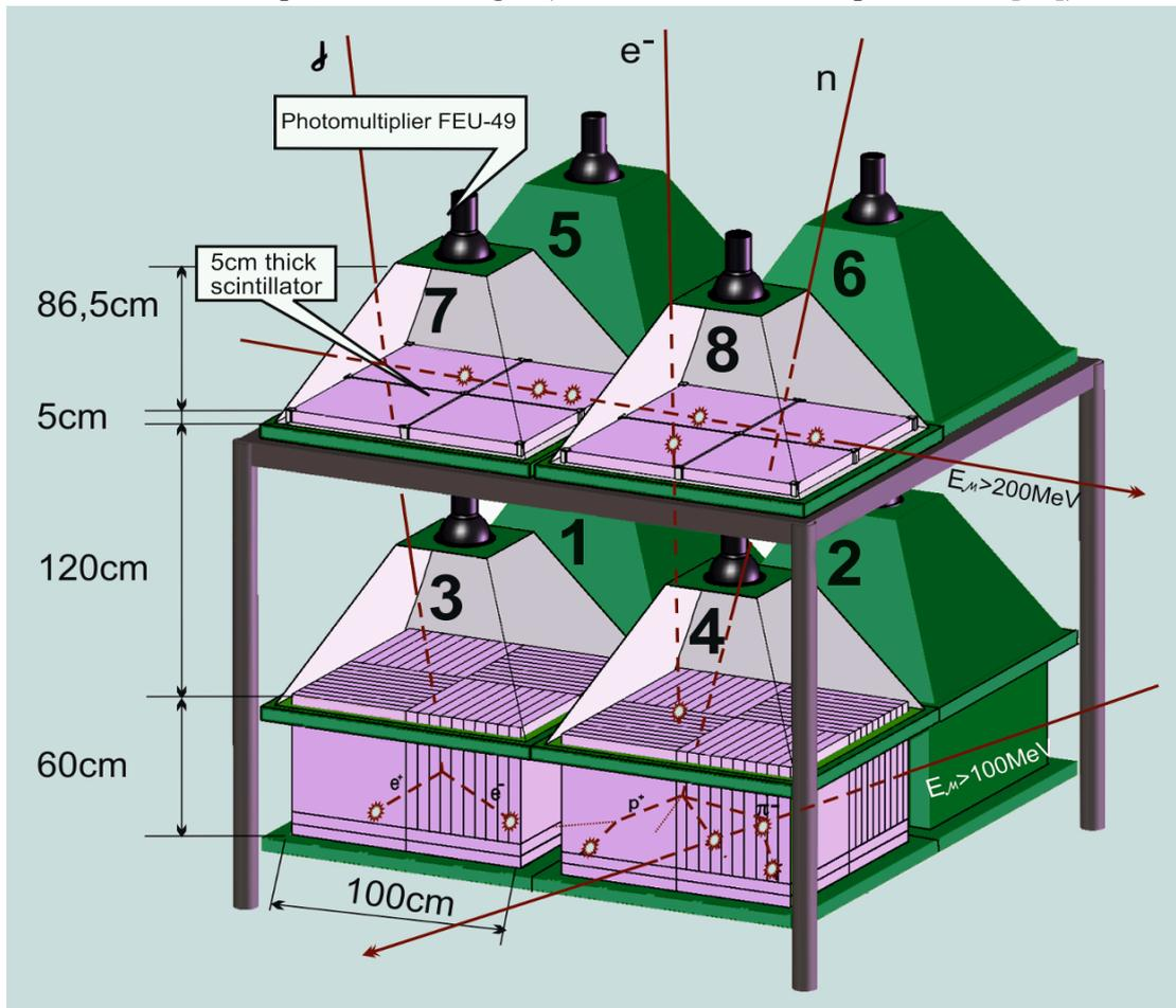
**Figure 7. Assembly of ASNT with a schematic view of the different particles traversing the detector. TGE electrons are registered by both upper and lower layers; gamma rays and neutrons – by invoking the veto option (no signals from the upper scintillators).**
