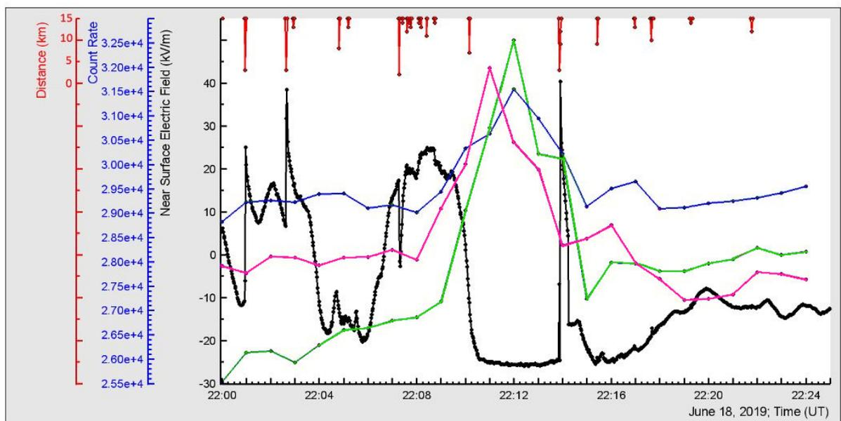
**Figure 3.** Time series of scintillator counters: SEVAN (blue), STAND1 (green), and STAND3 (magenta), see details in Table 1; disturbances of NSEF (black), and distances to lightning flash (red).
