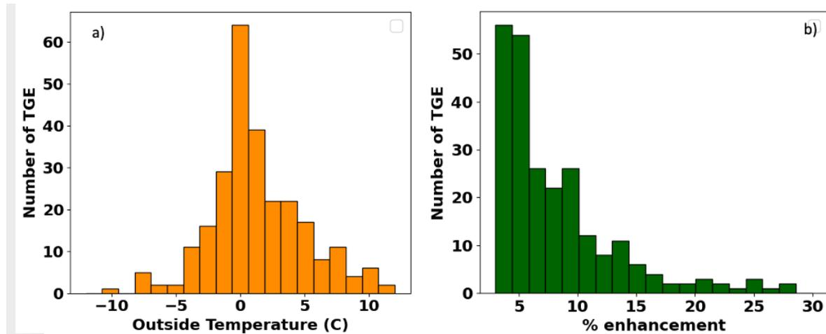
**Figure 5. a) The distribution of outside temperatures during TGEs; b) distribution of TGE significances by 3 cm thick plastic scintillator of STAND3 detector.**
