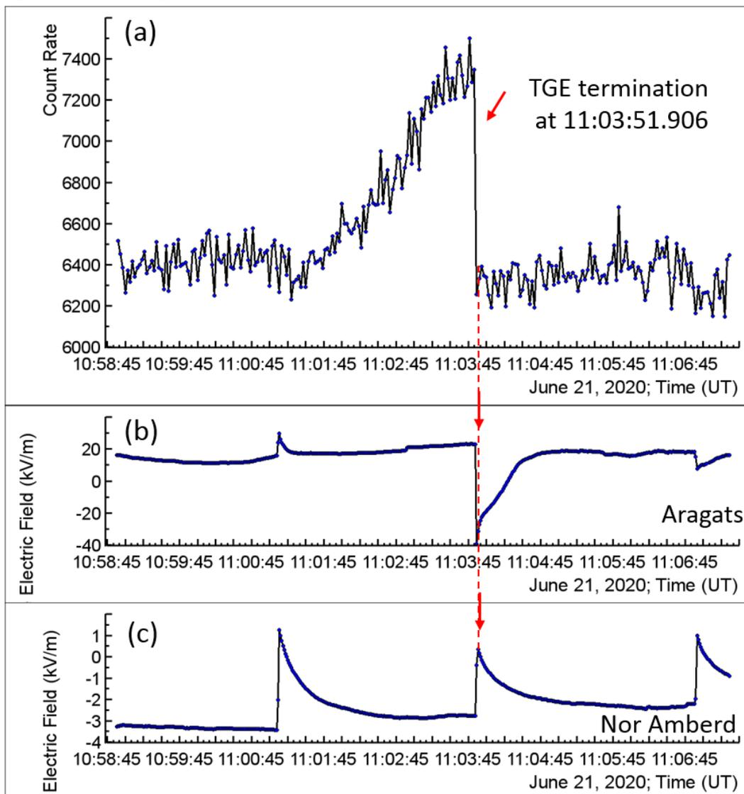
**Figure 6.** TGE terminated by a lightning flash that occurred at 11:03:51.906 on June 21, 2020. The upper panel (a) shows the count rate of the scintillation detector. Panels (b) and (c) show the NSEF measured at Aragats and Nor Amberd stations, respectively.
