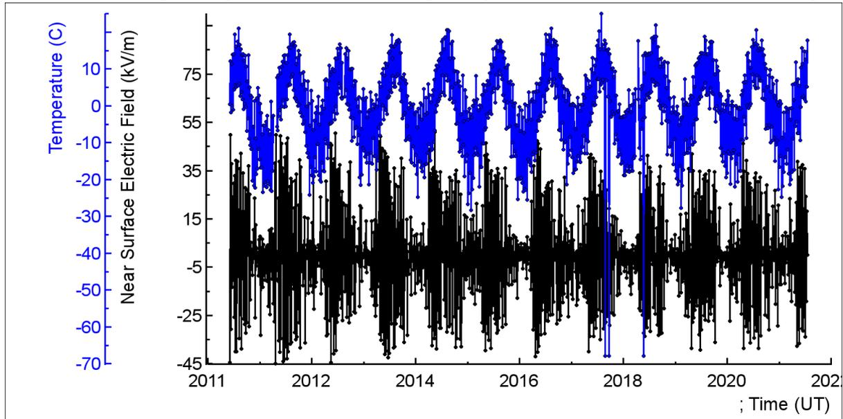
**Figure 1. Daily time series of the NSEF (electric mill EFM-100 by BOLTEK firm, black), and outside temperature (DAVIS weather station, blue)**
