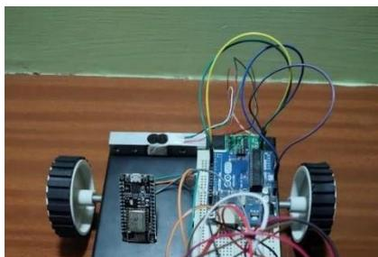
Figure 9. Load cell with Arduino UNO
