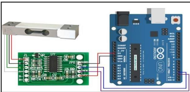
Figure 3. Arduino Uno with Load cell & Amplifier module
