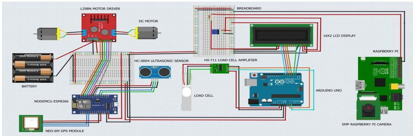
Figure 7. Circuit Diagram of proposed hardware
