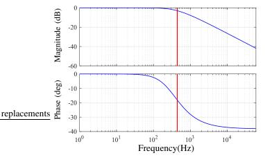
Fig. 1: Bode plot of the describing function of a HIGS of the form (1) with  $k_h = 1$  and  $\omega_h = 600\pi$  rad/s.
