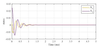
Fig. 5: Evolution of state trajectories of the nanopositioner plant under the control of a HIGS controller of the form (1) with  $k_h = 0.4939$  and  $\omega_h = 1.1705 \times 10^4$  rad/s
