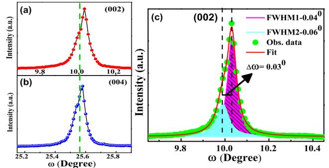
FIG. 4. (a)-(b) Rocking curve (RC) of  $(002)$  and  $(004)$  plane of crystal, dotted line shows the presence of kink. (c) Deconvoluted RC of  $(002)$  diffracting plane.
