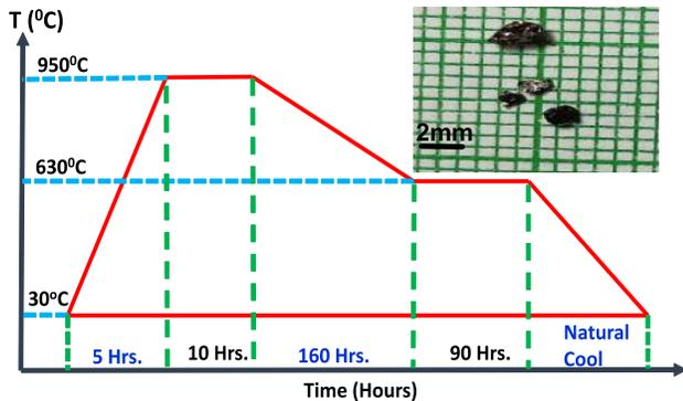
FIG. 1. Time-Temperature profile for the growth of DySb single crystal, along with cleaved crystals.
