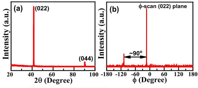
FIG. 3. (a)  $\theta$ - $2\theta$ , XRD scan of  $\{022\}$  planes. (b) Azimuthal  $\phi$ -scan of  $(022)$  plane.
