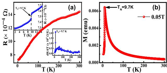
FIG. 5. (a) Variation of electrical Resistance ( $R$ ) as a function of temperature ( $T$ ). Upper inset: Enlarged view of RT data below 15 K showing transition point  $T_N$ . Lower inset:  $\frac{dR}{dT}$  data as a function of temperature. (b) Temperature dependence of magnetisation ( $M$ - $T$ ) in an applied field of 0.05 T.
