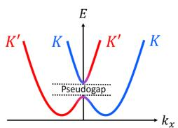
Figure 2. Schematic plots. (a) Rashba valley splitting in energy subbands of a graphene quantum wire (in the x-direction) with an in-plane electric field (in the y-direction), when intervalley scattering is excluded. (b) Opening of a pseudogap when intervalley scattering is included.
