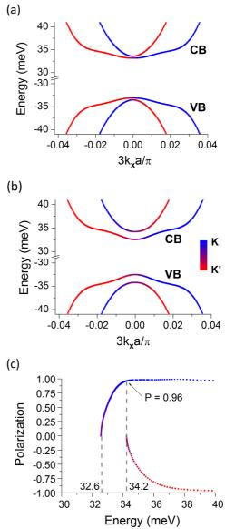
**Figure 8.** Subbands and polarization for the BLGbased Type-I filter configuration with  $W_1 = W_3 = 90$ Å,  $W_2 = 100$  Å,  $\Delta_1 = \Delta_3 = 116$  meV,  $\Delta_2 = 17$  meV,  $V_1 - V_3 = 70$  meV, and conduction band offset = 99 meV. (a) Conduction bands (CB) and valence bands (VB) in the quantum wire calculated by taking  $W_1 = W_3 = \infty$ . Blue curves: subbands of K pseudospin.
