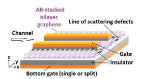
**Figure 3.** The structure of a proposed valley filter in BLG, where BLG is placed on a substrate and is implanted with scattering defects in parallel to the quantum wire channel. Two top gates are placed above BLG, and a (single or split) back gate is placed below the insulator substrate.
