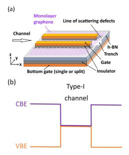
**Figure 7. (a)** The proposed structure of a valley filter in SLG/h-BN, where SLG is placed on a trenched h-BN substrate and is implanted with scattering defects in parallel to the quantum wire channel. Two top gates are placed above SLG, and a (single or split) back gate is placed below the insulator substrate. **(b)** Corresponding transverse band edge profile showing a Type-I channel. CBE: conduction band edge, and VBE: valence band edge.
