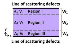
**Figure 4.** Top view of a valley filter, with Region II being the quantum wire channel, and Regions I and III being potential barriers.
