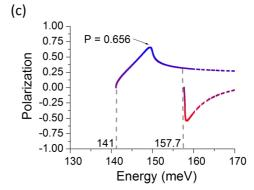
**Figure 9.** Subbands and polarization for the BLGbased Type-II filter configuration with  $W_1 = W_3 = 40$ Å,  $W_2 = 50$ Å,  $\Delta_1 = \Delta_3 = 149$  meV,  $\Delta_2 = 127$  meV,  $V_1 - V_3 = 80$  meV, and conduction band offset = 125 meV. (a) Conduction bands (CB) and valence bands (VB) in the quantum wire calculated by taking  $W_1$
