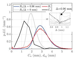
Fig. 9 Measured chord length distribution  $C_n$  and the resulting bubble size distribution as measured using the needles  $B_n$  compared to the bubble size distribution obtained via the camera  $B_c$ . Measured at z=3.4 m and V=0.55 Lm<sup>-1</sup>s<sup>-1</sup>
