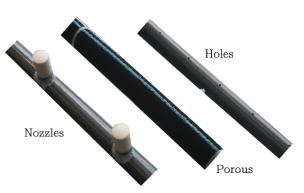
Fig. B2 The three different hoses used in the experiments
