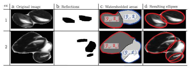
**Fig. 6** Illustration of the bubble cluster deconstruction algorithm. 2 examples have been given: example 1 shows an almost perfect fit, example 2 shows a less successful application of the algorithm. a) The original images. b) Recognition of the bubble reflections. c) Watershedded areas constructed using the reflections. The coordinates of the contours are shown. d) The resulting ellipses
