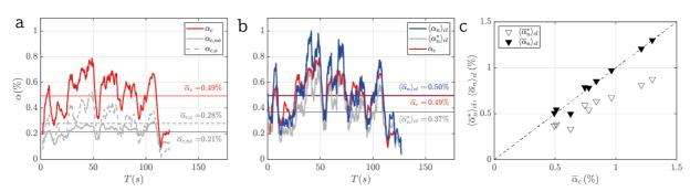
Fig. 7 a) Contribution of individual bubbles and bubbles in clusters to the void measured by the camera. b) Comparison of void fraction measured by the camera and by the electrical probes. c) Average uncorrected and corrected needle probe void fraction compared to the camera void fraction; the dashed line indicates the diagonal.
