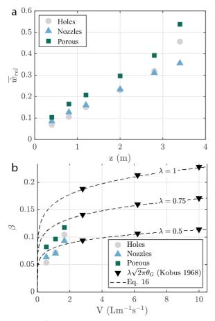
**Fig. 13** a) Top hat width of the three different hose types at  $V = 1.67 \,\mathrm{Lm^{-1}s^{-1}}$ . b) Spreading parameter for all hose types at varying gas flow rates compared to the relation given in Eq. 16 and experimental data of Kobus (1968)
