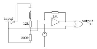
Fig. A1 The circuitry used by the needle probes, can be actuated either by a constant input(DC) or by an alternating input (AC)
