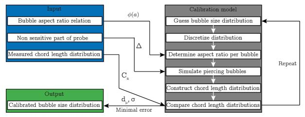
Fig. 4 Schematic of calibration algorithm
