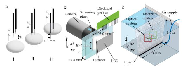
Fig. 3 a) Electrical probes, I a bubble approaches a set of double needles both needles are in full contact with water (signal 0 0), II Bubble encapsulates the tip of the longer needle (signal 1 0), III bubble left longer needle and encapsulates the shorter needle (signal 0 1). b) Optical system. c) Experimental setup with the bubble curtain hose, air supply, optical system and electrical probes
