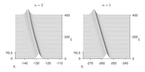
Figure 3: Solitary wave solutions over the periodic forcing. Parameters:  $\Delta = -2a$ ,  $x_0 = -\pi/2q$ , A = -1.
