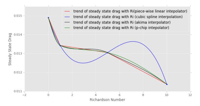
Fig 12 : Variation of steady state drag force with Richardson Number for the Lid Driven Cavity
