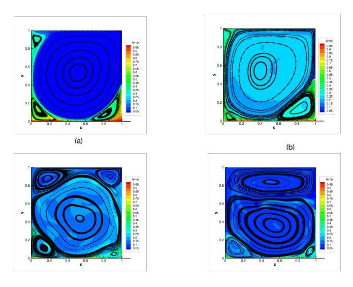
Fig 9 : Temperature Contours for (a) Ri = 0, (b) Ri = 1, (c) Ri = 5, (d) Ri = 10
