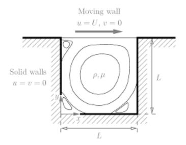
The top wall moves along the positive x-direction with a constant velocity of  $U_o$  and all the other walls are stationary. The walls are at some known reference temperature and the cavity is filled with water. The thermo-physical properties of the working fluid is assumed to be constant except the mass density which will vary according to the Boussinesq approximation. The fluid is taken to be
