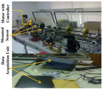
Fig. 7. Experimental setup of the intelligent fault signal simulator with data acquisition system IV. CONCLUSION
