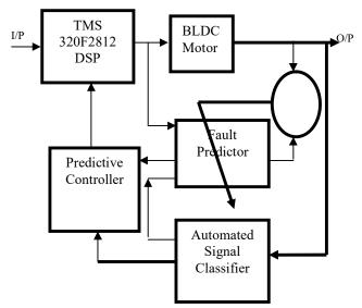
Fig. 3.Architecture of the proposed Intelligent Fault aware controller
