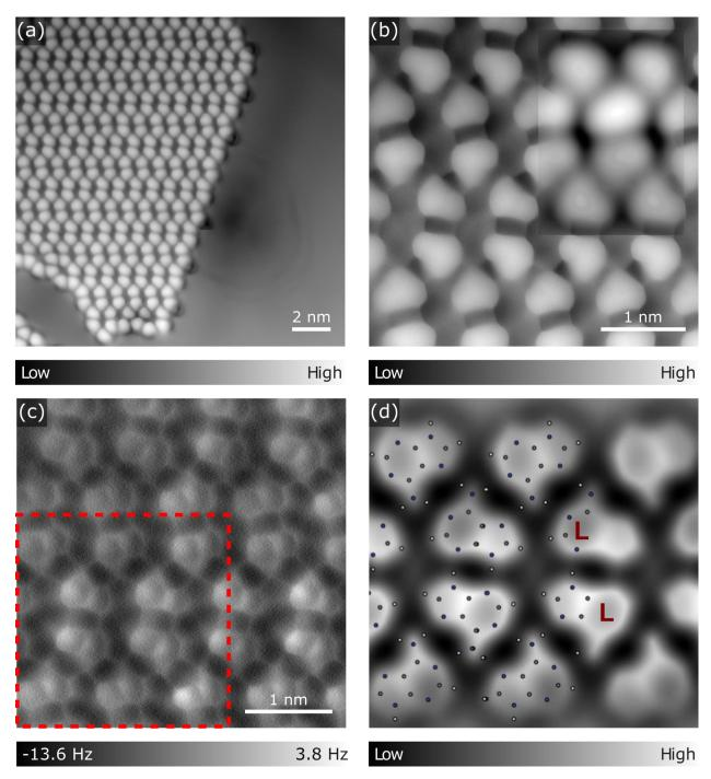
Figure 1: Self-assembly of adenine on Ag(111) probed by a CO-tip STM and AFM. (a) STM topography overview of an adenine island. Setpoint: 100 mV, 100 pA. (b,c) Zoomed-in STM topography of the island with a simulated STM image as an inset (b) and the corresponding constant-height AFM image (c). (d) Simulated AFM image with the overlaid molecular structure corresponding to the area marked in (c).
