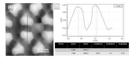
Figure S6: Example of the distance determination between the adenine rows after hydration at 200 K. Average over several line profiles yields 0.67 nm.
