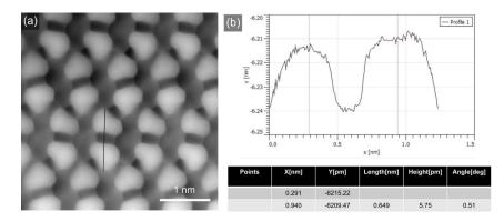
Figure S5: Example of the distance determination between the adenine rows before hydration. Average over several line profiles yields 0.65 nm.
