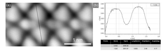
Figure S7: Example of the distance determination between the adenine rows after hydration at RT. Average over several line profiles yields 0.82 nm.
