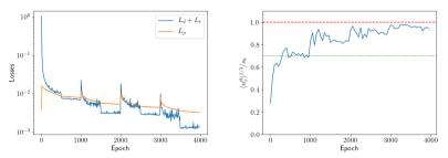
Fig. 3 PINN results for Experiment 2: (a) Evolution of the  $L_d + L_t$  and  $L_p$  lesses as a function of the training epoch. (b) Evolution of the centralized third order moment normalized by the target  $s_0$ , as a function of the training epoch. The dashed red line indicates the target value, while the dotted green line indicates the value of the seed field.
