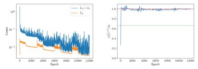
**Fig. 4** PINN results for Experiment 3: (a) Evolution of the  $L_d + L_t$  and  $L_p$  losses as a function of the training epoch. (b) Evolution of the centralized fourth order moment normalized by the target  $k_0$ , as a function of the training epoch. The dashed red line indicates the target value, while the dotted green line indicates the value of the seed field.
