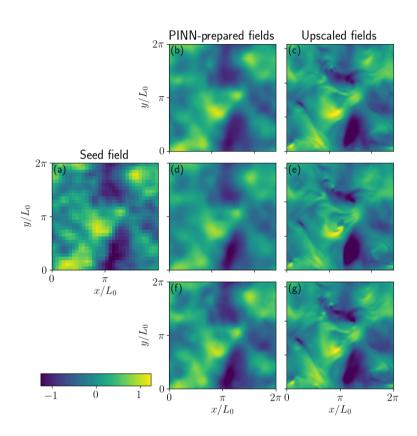
Fig. 2 Visualizations of a two-dimensional slice of (a) the seed (*u* velocity component), (b) the PINN output when imposing a mean velocity profile with (c) its corresponding nudgingupscaled field, (d) the PINN output with third order moment imposed and (e) upscaled field, and (f) the PINN output with fourth order moment imposed and (g) upscaled field. All slices correspond to time  $t = 1.125T_0$  and  $z = \pi/L_0$ .
