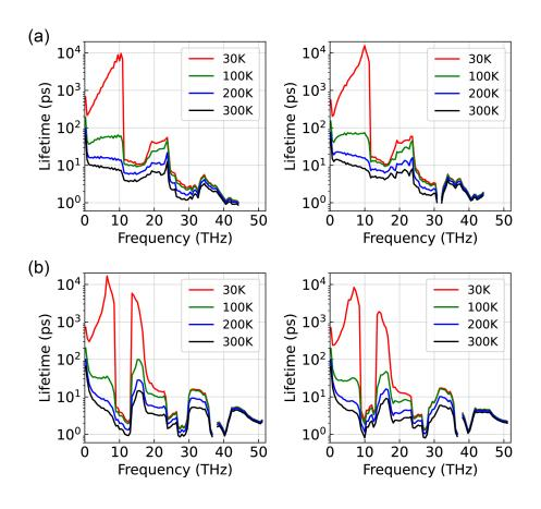
Fig. 7. The phonon lifetime distribution of g-BN monolayer under (a) tensile and (b) compressive strain of 5% along the zigzag (left panel) and armchair directions (right panel) at four different temperatures.
