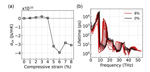
Fig. 8. (a)  $\alpha_{zx}$  of g-BN at 30 K under 0~8 % compressive strain along the zigzag direction and (b) their phonon lifetime. The lines are colored in gradation from black to red in an interval of 1% strain.
