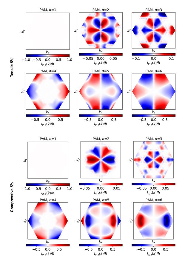
Fig. S5. Mode-specific PAM textures of g-BN under tensile and compressive strains of 5% along the armchair direction. No PAM exists for  $\sigma$ =1.
