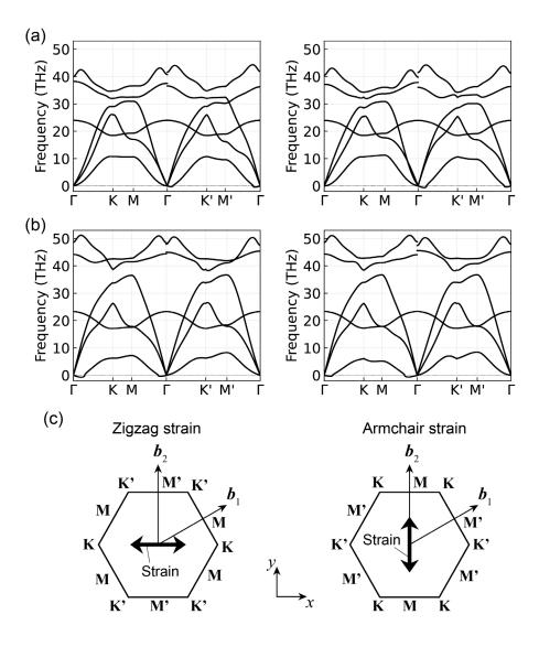
**Fig. 5. Phonon band structures of g-BN under strain.** (a) Tensile and (b) compressive strain of about 5% along the zigzag (left panel) and armchair directions (right panel). (c) Strain directions and high-symmetry points in the Brillouin zone.
