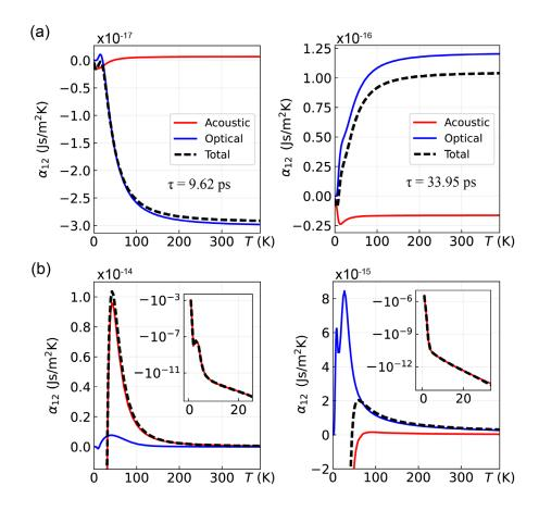
Fig. 2. PAM response tensor  $\alpha_{xy}$  of AlN (left panel) and GaN (right panel). (a) Constant phonon lifetime ( $\tau$ = 9.62 and 33.95 ps) and (b) mode-specific phonon lifetime are used. The contributions of acoustic (red) and optical modes (blue), and the total (black dashed) are plotted. Insets in (b) used logarithmic scale.
