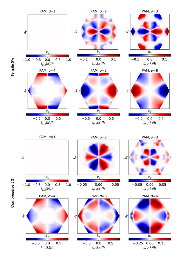
Fig. S4. Mode-specific PAM textures of g-BN under tensile and compressive strains of 5% along the zigzag direction. No PAM exists for  $\sigma$ =1.
