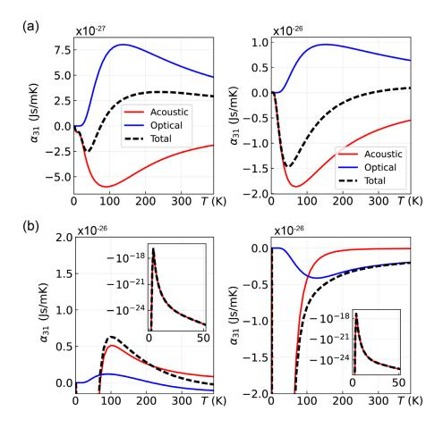
Fig. 6.  $\alpha_{zx}$  of g-BN under (a) tensile and (b) compressive strain of 5% along the zigzag (left panel) and armchair directions (right panel). The acoustic (red), optical modes (blue) contribution, and the total (black dashed) are plotted. Insets in (b) are the logarithmic plot. The legends are the same as in Fig. 2.
