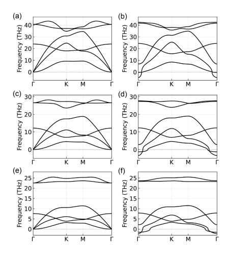
Fig. S6. Harmonic phonon band dispersion of (a) g-BN, (b) g-AlN, and (c) g-GaN. Left panel, first-principles calculations and right panel, the dynamical matrix model.
