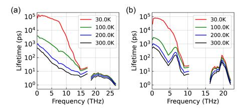
**Fig. 3. The phonon lifetime distribution of (a) AlN and (b) GaN.** Lifetime at each frequency is averaged over a frequency interval of ~0.13 THz.
