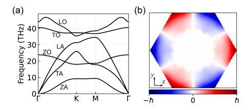
**Fig. 4. (a) Phonon band structure and (b) PAM texture of the fourth branch of g-BN.** The phonons at the K-point of the left panel in (a) are ZA, ZO, TA, LA, LO, and TO modes in ascending order in frequency.
