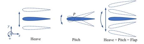
Figure 3: The motions of hydrofoil.
