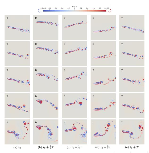
Figure 12: Snapshot series of the motion of active hydrofoil and its wake in one cycle  $(St_A=0.08(1^{st}\text{ row}), 0.12(2^{nd}\text{ row}), 0.16(3^{rd}\text{ row}), 0.24(4^{th}\text{ row}), 0.44(5^{th}\text{ row}), \Delta x = \frac{1}{1280}\text{ m}$ . The force status is marked in the top left corner, where D is for drag and T is for thrust.).
