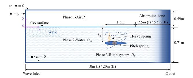
Figure 6: The schematic diagram of the passive hydrofoil simulation.
