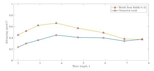
Figure 13: The comparison between the experiment (the upper line) and passive hydrofoil simulation ( $\Delta x = \frac{1}{160}$  m.)
