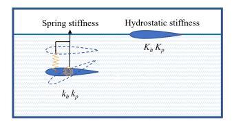
Figure 8: The heave and pitch spring stiffness (left) and the hydrostatic stiffness of the foil itself (right).
