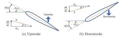
Figure 4: The illustration for the effective AOA  $\alpha_{eff}$  of flapping hydrofoil in uniform flow ( $\frac{dh}{dt}$  is the heave velocity, V is the velocity of the stream relative to the hydrofoil.).
