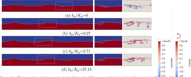
Figure 18: The snapshots of the passive hydrofoil under different non-dimensional pitching spring stiffness  $k_p/K_p$  (wavelength=3.75 m,  $t_0$  = 8.99 sec). The series of snapshots on the left shows the Heaviside fields, while those on the right show the zoomed-in Heaviside and vortex fields.
