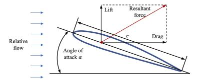
Figure 7: The forces on the foil facing flows.
