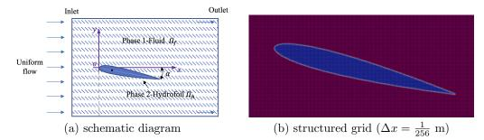
Figure 9: A schematic diagram (left) and partial structured grid (right) of the simulation for the fixed hydrofoil in uniform flow.
