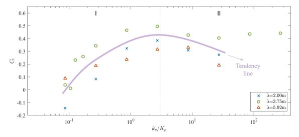
Figure 17: The thrust coefficient  $C_t$  of the passive hydrofoil with different non-dimensional pitch stiffness  $k_p/K_p(\Delta x = \frac{1}{160} \text{ m})$ .
