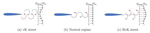
Figure 5: The illustration for the drag-to-thrust wake transition of flapping hydrofoil.
