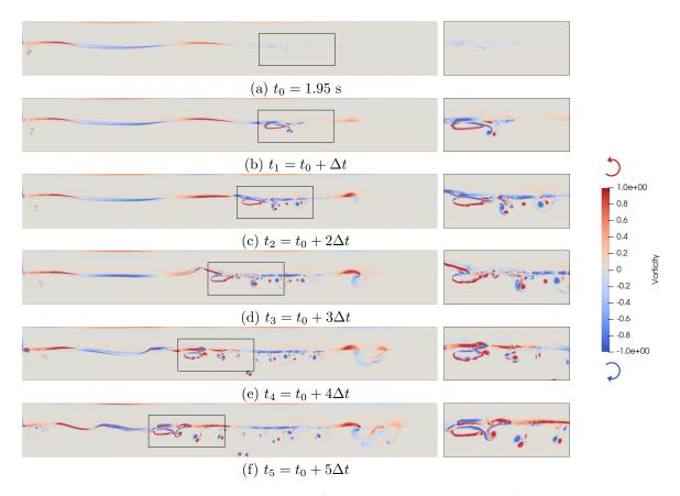
Figure 19: The position of the passive hydrofoil in wave (wavelength=3.75 m, time interval  $\Delta t = 1.70$  sec is the wave period). The series of snapshots on the right are the zoomed-in parts.
