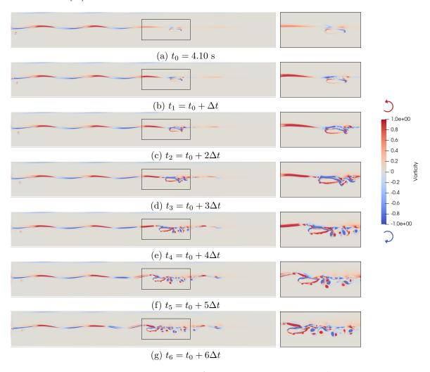
Figure 14: The position of the passive hydrofoil in wave (wavelength=2.00 m, time interval  $\Delta t = 1.15$  sec is the wave period). The series of snapshots on the right are the zoomed-in parts.
