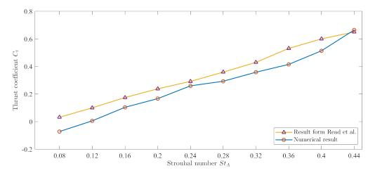
Figure 11: The comparison between the experiment (the upper line) and active hydrofoil simulation ( $\Delta x = \frac{1}{1280}$  m).
