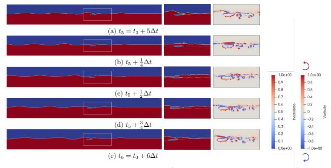
Figure 15: The position of the passive hydrofoil in one wave period (wavelength=2.00 m,  $t_0 = 4.10$  sec, time interval  $\Delta t = 1.15$  sec is the wave period). The series of snapshots on the left shows the Heaviside fields, while those on the right show the zoomed-in vortex fields. The dash lines are the chord lines.
