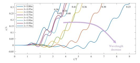
Figure 16: The non-dimensional displacement  $x/\lambda$  of the passive hydrofoil with time over wave period t/T facing different waves  $(\Delta x = \frac{1}{160} \text{ m})$ .
