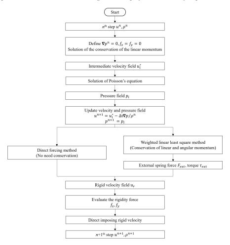
Figure 1: The flow chart of the 'one-fluid' framework.
