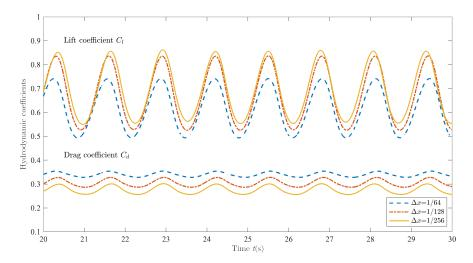
Figure 10: Validation of convergence of fixed hydrofoil facing uniform flow simulations.
