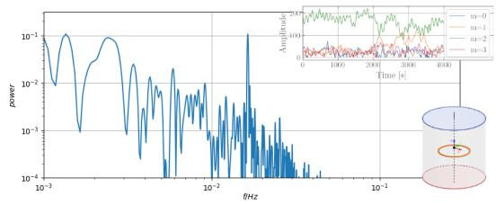
Figure 3: Frequency spectrum of the m=2 mode of the radial velocity measured at sensor points on the orange ring. Note the clear peak at the modulation frequency of 0.01818 Hz.
