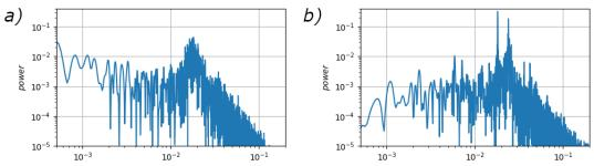
Figure 6: Frequency spectrum of the mean helicity within -0.09 m  $\leq$  x  $\leq$  0.0 m for a) a pure RBC and b) a RBC exposed to an additional m=2 forcing with 27.6A and 25 Hz and a modulation frequency of  $f_{LSC}$ =0.01818Hz.
