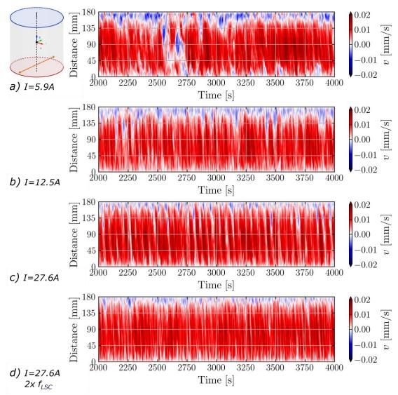
Figure 7: Comparison of flow speeds taken from a sensor path (orange line) over time for different electromagnetic forces produced by different currents (f=25 Hz) and a modulation frequency  $f_{LSC}$ =0.01818 Hz (a,b,c) and 0.03636 Hz (d).
