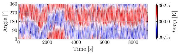
Figure 5: Time series of the temperature distribution over angle for a RBC combined with a  $60^{\circ}$  turned m=2 forcing (30A, 25Hz) and a modulation frequency of  $f_{LSC}$ =0.01818Hz. At t=0, the RBC is already fully developed (the prior transient over 3000 s is not shown here).
