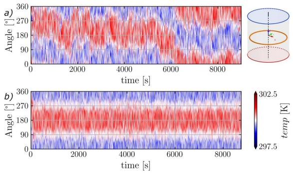
Figure 4: Time series of the temperature distribution over angle taken from the orange sensor ring for a) a pure RBC and b) a RBC combined with a m=2 forcing (30A, 25Hz) and a modulation frequency of  $f_{LSC}$ =0.01818Hz. At t=0, the RBC is already fully developed (the prior transient over 3000 s is not shown here).
