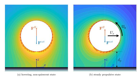
FIG. 1: (a) Hovering and (b) self-propelling states of an isotropic phoretic particle near a rigid wall. The particle-wall separation is set by a balance between the external force  $\mathbf{F}^{ext}$ , and the solute-accumulation-induced repulsive force  $\mathbf{F}^{H}$ .
