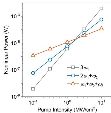
**Fig. 5.** The power dependence of nonlinear third-order frequency mixing processes including THG ( $3\omega_1$ ), dFWM ( $2\omega_1 + \omega_2$ ), and non-dFWM ( $\omega_1 + \omega_2 + \omega_3$ ) on the power of the  $\omega_1$  pump.
