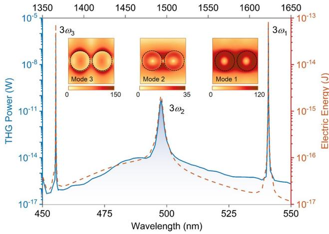
**Fig. 3.** The THG power (solid) and electric energy inside the nanodisk dimers (dashed) of the metasurface under  $y$ -polarized oblique incidence. Insets are the enhancement of electric field intensity ( $|E|/|E_0|$ ) at the fundamental wavelengths of the three quasi-BIC resonances.
