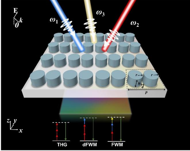
**Fig. 1.** The schematic of the designed metasurface consisting of a square array of silicon nanodisk dimers, simultaneously illuminated by three pump beams termed as  $\omega_1$ ,  $\omega_2$ , and  $\omega_3$  in the near-infrared regime to generate a variety of new visible frequencies. The unit cell is indicated by a dotted square. The bottom inset illustrates the schematic energy diagrams of the nonlinear optical processes that occur simultaneously to generate visible emissions.
