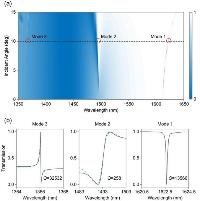
**Fig. 2.** (a) The transmission of the metasurface as a function of wavelength and incident angle. As seen, the resonances corresponding to the excitations of the three quasi-BIC modes show narrow linewidth, when the modes evolve from the perfect BIC to quasi-BIC. (b) The simulated (solid) and theoretical (dashed) transmission spectra of the metasurface under  $y$ -polarized oblique incidence of  $10^\circ$  in the vicinity of the three quasi-BIC resonances.
