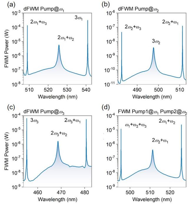
**Fig. 4.** The nonlinearly generated visible signals originating from optical frequency mixing under  $y$ -polarized oblique incidence when the multiple beams simultaneously pump the metasurface. (a)-(c) Two pump beams are considered with one at a fixed wavelength of  $\omega_1$ ,  $\omega_2$ , and  $\omega_3$ , respectively. (d) Three pump beams are considered with two fixed wavelengths at  $\omega_1$  and  $\omega_2$ .
