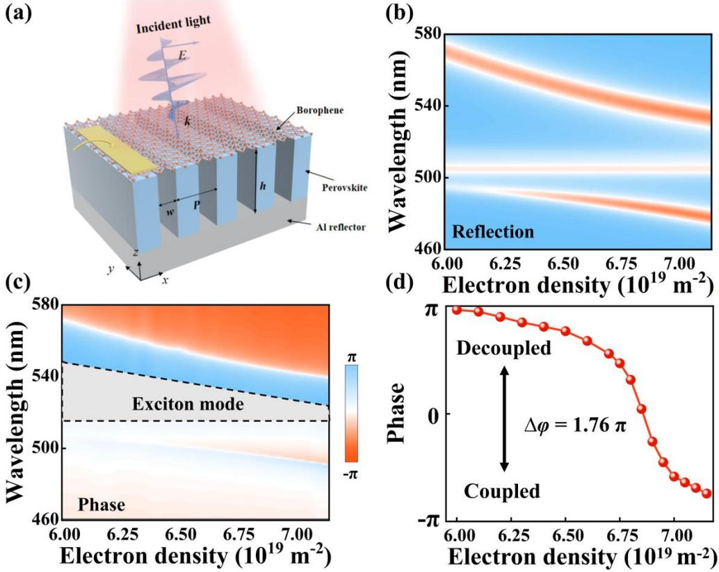
Fig. 3. (a) The schematic of the phase modulator. The reflection (b) and phase (c) dispersion curves as a function of the electron density  $n$ . (d) Calculated phase at 545 nm with a varied electron density  $n$ .
