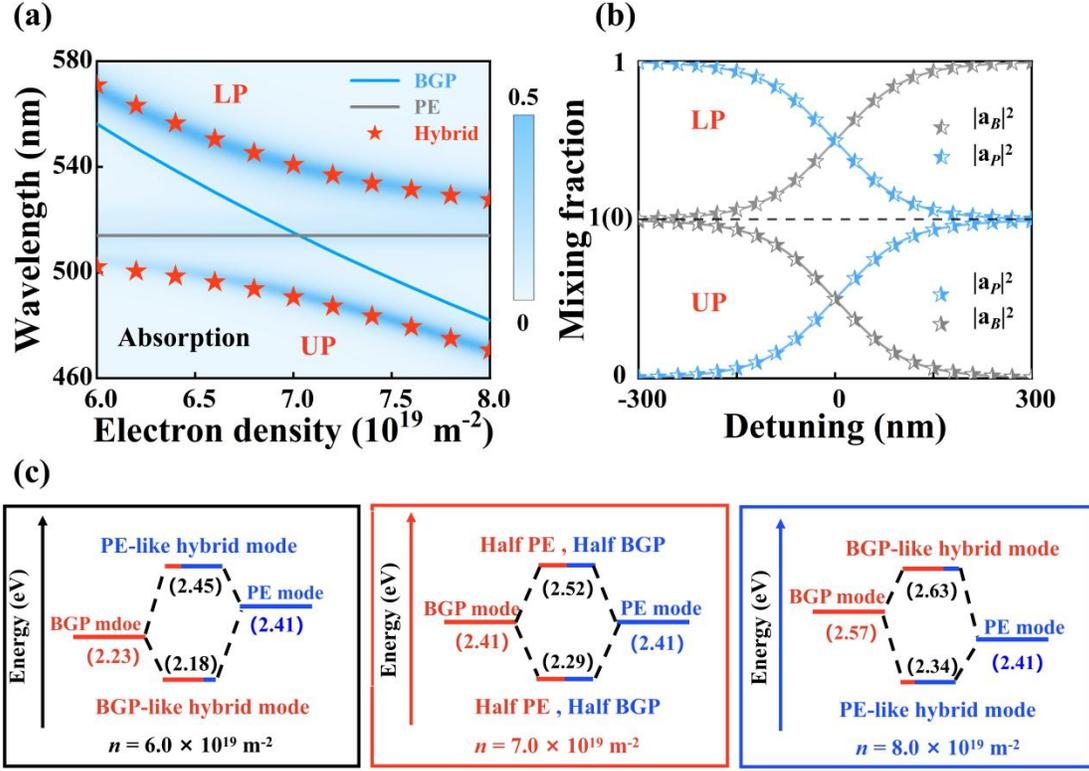
Fig. 2. (a) The hybridized modes dispersion curves with a varied electron density  $n$  and theoretically analyzed hybrid modes (stars), original BGP mode (blue line), and PE mode (grey line) mode. (b) The mixing fraction of the upper and lower dispersion curves as a function of detuning. (c) The energy schematic cases in Fig. 2(a).
