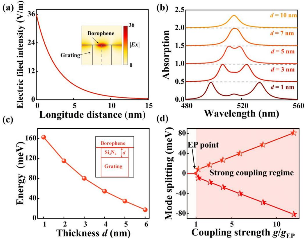
Fig. 4. (a) The normalized electric field intensity fetched from the grey dotted line in the insert as a function of longitude distance. (b) The absorption spectra evolutionary process with the increase of dielectric layer thickness  $d$ . (c) The splitting energy as a function of dielectric layer thickness  $d$ . The insert is the side view of the structure. (d) Calculated mode splitting with varied coupling strength.
