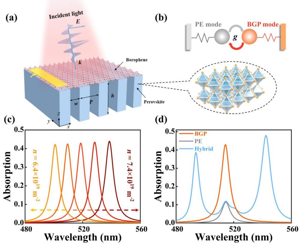
Fig. 1. (a) Schematic of the proposed plasmon-exciton hybridized system. (b) Theoretical coupled oscillator model. (c) The absorption spectra as a function of varied electron density  $n$ . (d) The absorption spectra of the borophene guiding plasmon, perovskite exciton, and hybridized modes.
