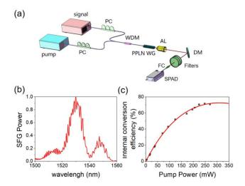
Fig. 2. (a) Experimental setup. PC, polarization controller; WDM, wavelength division multiplexer; WG, waveguide; AL, aspherical lens; DM, dichroic mirror; Filters, including a longpass filter, a shortpass filter, two bandpass filters, and an etalon; FC, fiber coupler; SPAD, silicon single-photon avalanche photodiode. (b) SFG tuning curve. (c) measured SFG conversion efficiency versus pump power (solid square), and the sin<sup>2</sup>() fitting curve.
