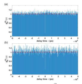
Fig. 5 Heralded self-correlation function  $g_{H}^{(2)}(\tau)$  for (a) signal-signal and (b) SF-SF.
