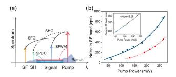
Fig. 3 (a) The main noise processes induced by a strong pump field in a QFC chip. (b) The total on-chip NCR (blue line, square) and the SHG-SPDC induced on-chip NCR (red dotted line, triangle) in the SF band over a detection bandwidth of 0.09 nm in linear coordinate. The inset shows the total on-chip NCR at high pump power in the logarithmic coordinates with the same detection bandwidth and the slope at 240 mW (red short dash).
