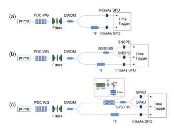
Fig. 4 The second-order correlation function measurement setups of the (a) photon pair, (b) heralded single-photon source, and (c) QFC of
