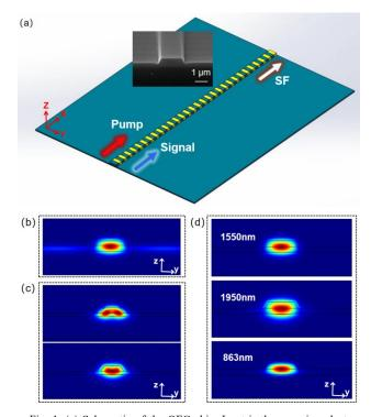
Fig. 1. (a) Schematic of the QFC chip. Inset is the scanning electron microscopy image of the fabricated waveguide. (b) Simulated profiles for the lateral leakage mode at 1550 nm. (c) Simulated profiles for hybrid modes at 1950 nm. (d) Simulated profiles for the quasi-TM mode of the signal, pump, and SF. The LN thickness, top width, ridge height, and sidewall angle are 800 nm, 1.8  $\mu$ m, 422 nm, and 60°, respectively.
