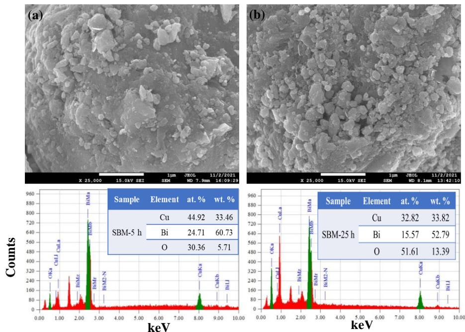
**Fig. 2** – SEM micrographs and EDX spectra of the (a) SBM-5 h and (b) SBM-25 h samples.
