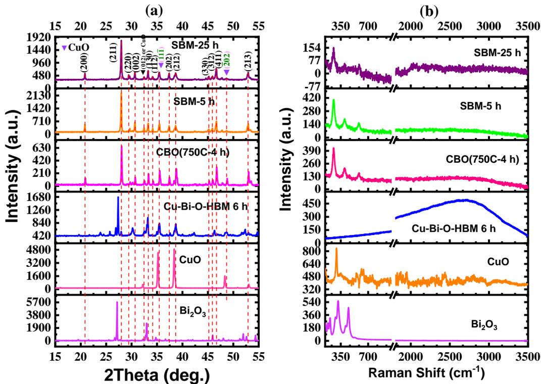
**Fig. 1** – (a) X-ray diffraction (XRD) patterns and (b) room temperature Raman spectra of the samples along with the raw materials CuO and Bi<sub>2</sub>O<sub>3</sub>.
