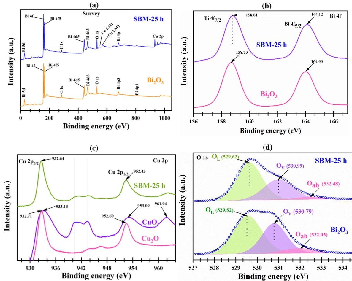
**Fig. 3** – (a) XPS spectra of  $CuBi_2O_4$  and  $Bi_2O_3$  showing regions for the core level of (b) Bi 4f, (c) Cu 2p, and (d) O 1s.
