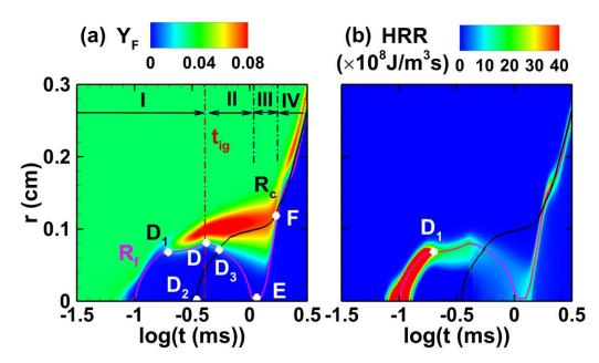
Fig. 5. r - t diagram of (a) fuel vapor mass fraction and (b) heat release rate with  $\phi_g = 0.3$ ,  $\phi_l = 1.7$ ,  $d_0 = 15 \ \mu \text{m}$ .  $E_{ig} = 1.76 \ \text{mJ}$ . Solid line: trajectories of the flame front (pink) or evaporation completion front (black).
