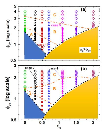
Fig. 11. Regime map of ethanol spray ignition regime in  $\phi_g - \phi_{ov}$  space: (a)  $d_0 = 5 \ \mu m$  and (b)  $d_0 = 15 \ \mu m$ . Orange dash-dotted line: regime boundary. Black dashed line:  $\phi_g = \phi_{ov}$ . Black dash-dotted line: ignitability limit of ethanol sprays. Green symbols: pure ethanol sprays from [10].
