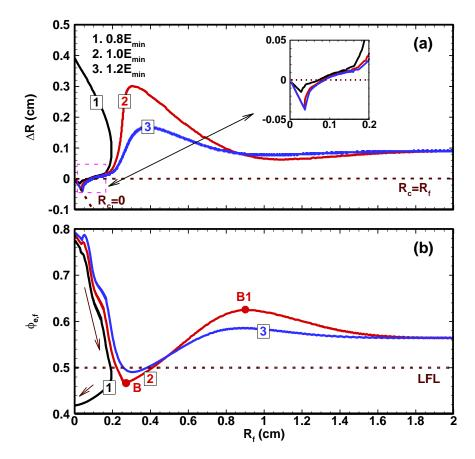
Fig. 4. Change of (a) front distance and (b) flame ER in case 1 with different ignition energies. The arrow in (b) indicates kernel propagation direction.
