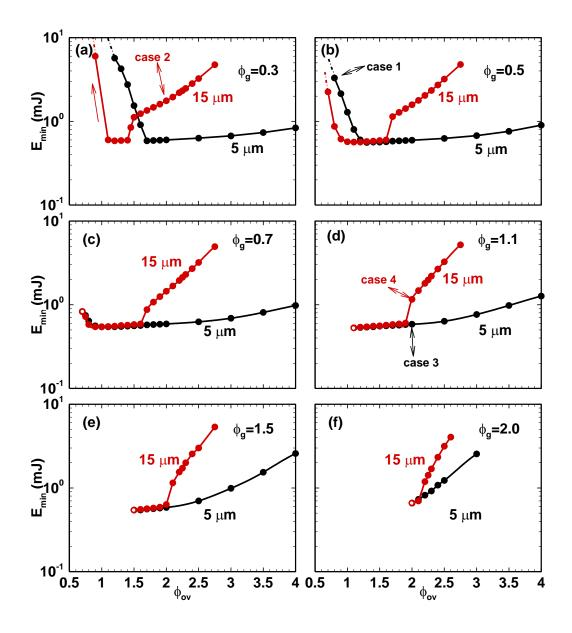
Fig. 10. Minimum ignition energy as a function of overall ER with different background gas ERs: (a)  $\phi_g = 0.3$ , (b)  $\phi_g = 0.5$ , (c)  $\phi_g = 0.7$ , (d)  $\phi_g = 1.1$ , (e)  $\phi_g = 1.5$ , (f)  $\phi_g = 2.0$ . Hollow symbol: gaseous flame under the corresponding background gas ER, i.e.,  $\phi_{ov} = \phi_g$ .
