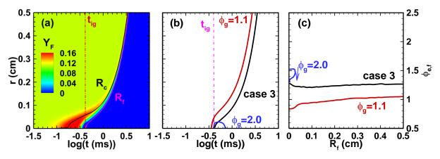
Fig. 8. (a) r - t diagram of fuel vapor mass fraction with  $\phi_g = 1.1$ ,  $\phi_l = 0.9$ , and  $d_0 = 5 \ \mu m$  (case 3). (b) Flame trajectories and (c) flame ER in case 3 and two gaseous flames with ER = 1.1 and 2.0.  $E_{ig} = 0.585 \text{ mJ}$ .
