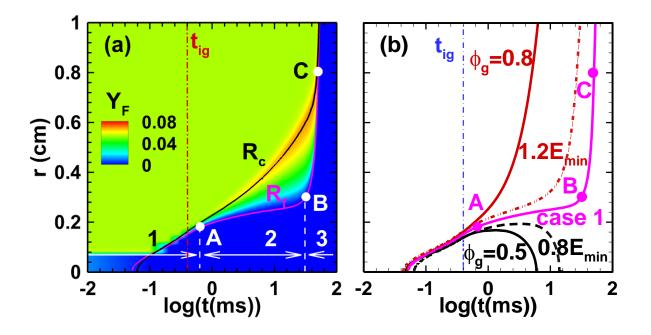
Fig. 2. (a) r - t diagram of fuel mass fraction with  $\phi_g = 0.5$ ,  $\phi_l = 0.3$ , and  $d_0 = 5 \ \mu m$  (case 1, spray flame).  $E_{ig} = E_{min} = 3.3 \text{ mJ}$ . (b) Flame trajectories of case 1 with different ignition energies. Gaseous flames with ER = 0.5 and 0.8 are added for comparison.
