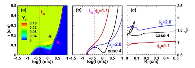
Fig. 9. (a) r - t diagram of fuel vapor mass fraction with  $\phi_g = 1.1$ ,  $\phi_l = 0.9$ , and  $d_0 = 15 \ \mu m$  (case 4). (b) Flame trajectories and (c) flame ER in case 4 and two gaseous flames with ER = 1.1 and 2.0.  $E_{ig} = 1.16 \text{ mJ}$ .
