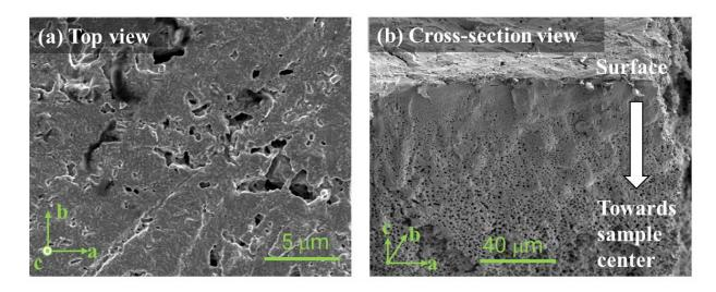
**Figure 1** Microstructure of a reduced single-crystalline cubic-Fe<sub>1-x</sub>O imaged by using SEM after partial reduction at 700°C for 2 hours under a H<sub>2</sub> flux of 30 L/h (a) Top view and (b) Cross-section view. The surface exposed to the reducing H<sub>2</sub> environment is perpendicular to the c direction.
