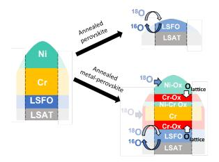
Figure 5: Conceptual schematic of the diverse oxygen transport pathways and reactions, highlighting OE between lattice oxygen in LSFO and  ${}^{18}O_{2(g)}$  coupled with oxidation of the metallic layers. Vertical dashed lines denote the conceptual field of view captured by APT; we hypothesize that the oxidation and passivation of the Cr could have also occurred over the exposed tip surfaces outside the field of view (i.e., more translucent regions at the shanks).
