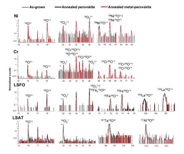
Figure S3: Isotopic analyses of key O ionic and isotopic species in a) Ni, b) Cr, (c) LSFO, and (d) LSAT phases. Peaks are labelled with their relevant ionic species that are present. Each range is normalized to the dominant <sup>16</sup>O isotope, to effectively measure changes in <sup>18</sup>O concentrations from the as-grown to perovskite and metal-perovskite annealed specimens. Potential PMI are identified in some cases, as denoted by multiple ionic species associated with a single peak.
