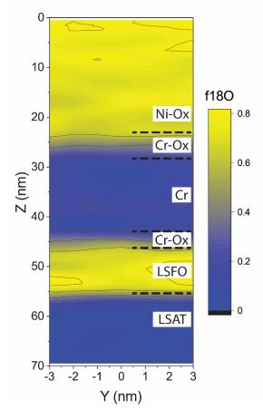
Figure 4: 2D heat map showing the oxygen isotopic composition across the annealed metal-perovskite specimen.
