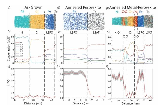
Figure 2: APT reconstructions, elemental profiles, and  $f^{18}O$  for the (a-c) as-grown vs. (d-f) annealed perovskite vs. (g-i) annealed metal-perovskite specimens. Shading is used to highlight the uncertainty associated with the counting statistics ( $1\sigma$ , see *Methods*).
