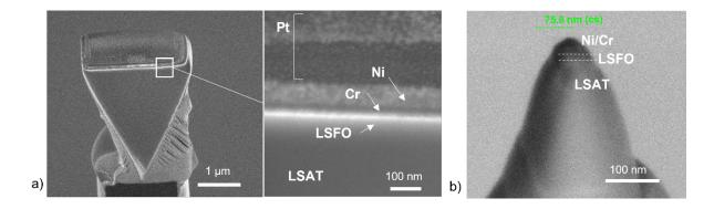
Figure S1: FIB-SEM preparation of APT tip from the Ni-Cr-LSFO-LSAT stack. Sample preparation is typical for an APT specimen; however, these SEM images are provided for additional context of capping scheme (a) before and (b) after tip sharpening.
