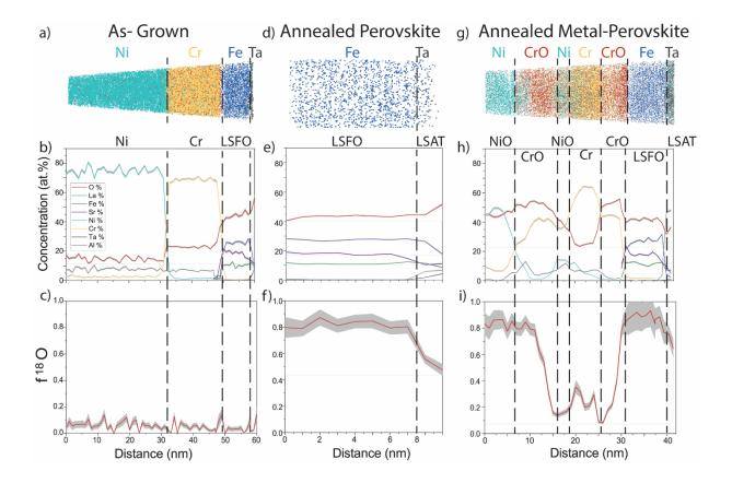
Figure S5. Analyses from additional APT tips with APT reconstructions, elemental profiles, and f<sup>18</sup>O for the as-grown vs. annealed perovskite vs. annealed metal-perovskite specimens. Shading is used to highlight the uncertainty associated with the counting statistics.
