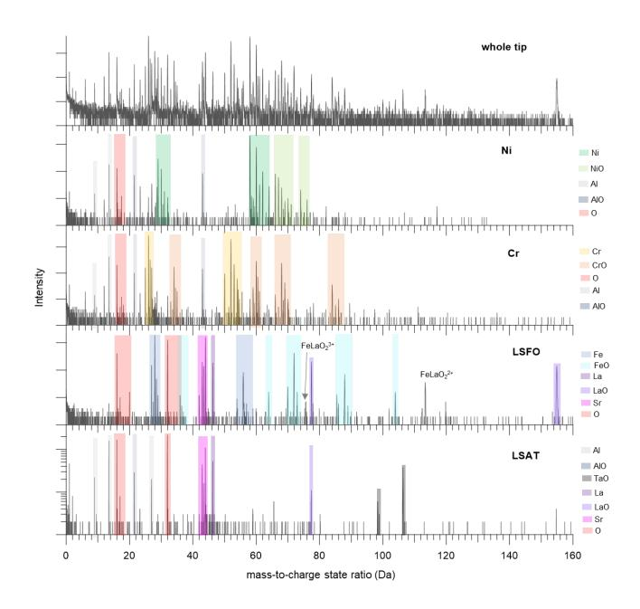
Fig S2: Mass spectra from as-grown specimen highlighting multi-elemental and isotopic nature of the heterostructure. Ion species were determined through analyses isolating the bulk in each layer. Dominant, general ionic species are labelled. Intensity is log-scale.
