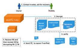
Fig. 2: The architecture of the proposed key recovery algorithm.
