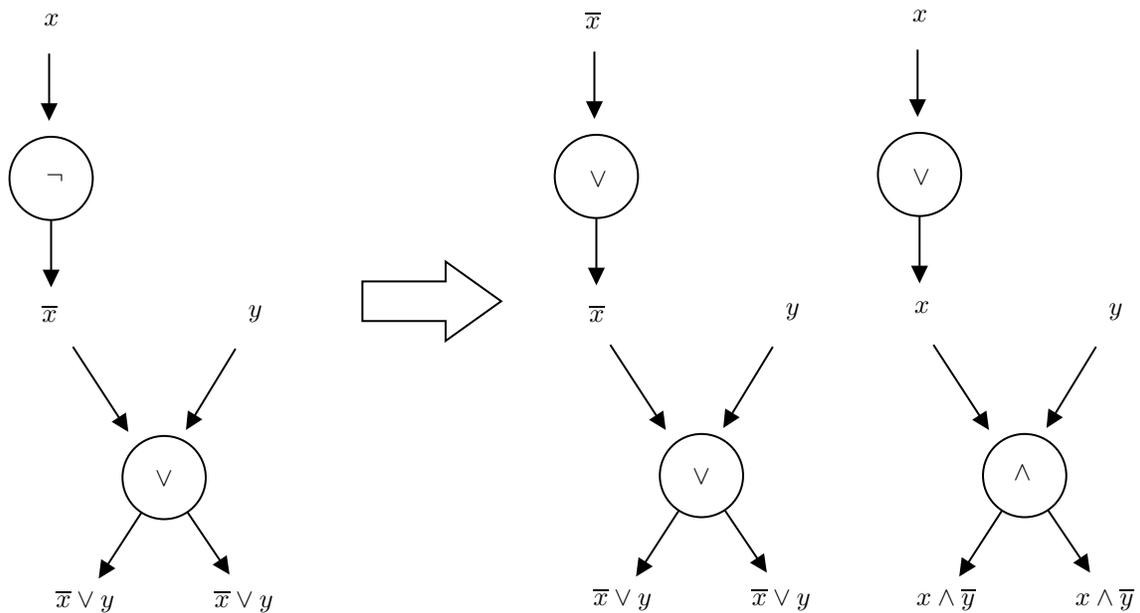
Figure 22: NOT gadget wiring for circuit simulation using gates from  $\mathcal{G}_m$ . In this case a NOT gate is connected to an OR gate in the original circuit. Copies of the NOT gate in the circuit performing simulation are connected to the copies of the OR gate switched: positive part is connected to negative part of the OR gate and viceversa.
