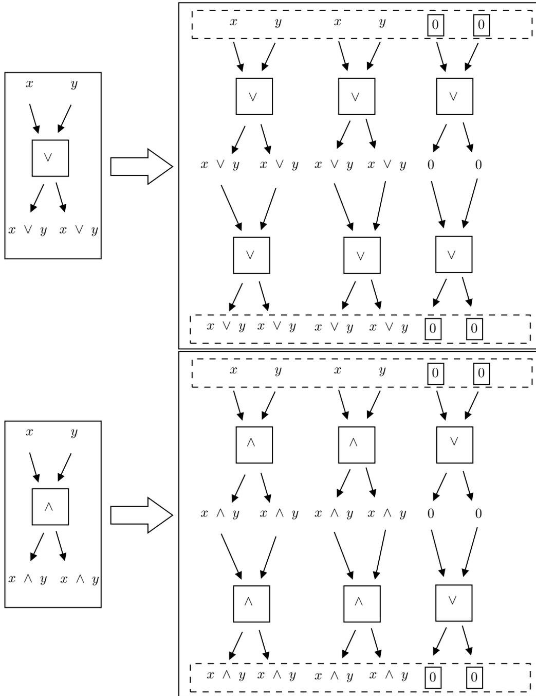
Figure 25: Block gadgets for simulating fanin 2 fanout 2 AND/OR gates using only gates in  $\mathcal{G}_{m,2}$ . Squared zeros represent the amount of zeros that can be used as inputs for the same block.
