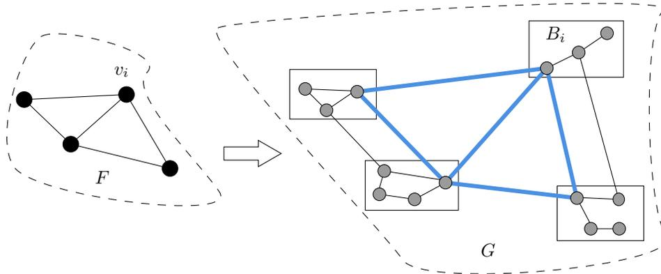
Figure 8: Scheme of one-to-one block simulation. In this case, network  $F$  is simulated by  $G$ . Each node in  $F$  is assigned to a block in  $G$  and state coding is injective. Observe that blocks are connected (one edge in the original graph may be represented by a path in the communication graph of  $G$ ) according to connections between nodes in the original network  $F$ . These connections are represented by blue lines
