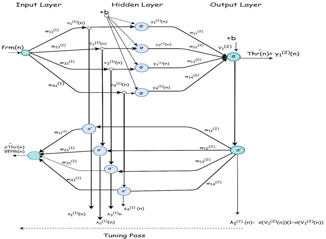
Figure 1. Flow chart of the proposed machine learning approach consisting of tuning pass, which depicts the derivation of the local gradients and the gradient for frame size adjustment.
