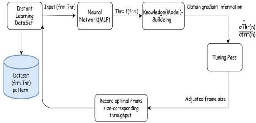
Figure 2. Basic components and flow of the proposed ML model
