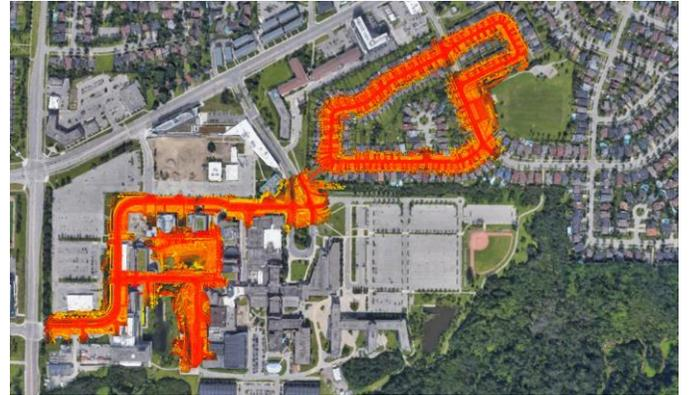
Fig. 4: PCL-map from 1st experiment aligned to Google Earth Map (Bird's Eye View)
