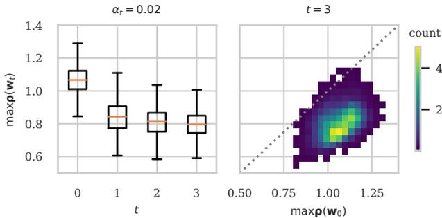
Fig. 1. Comparison with *Default OSPF* in 12,000 samples from the 4 real-world topologies of Table I. Left: Evolution of the maximum link utilization (y-axis) per optimization step with RBB (x-axis).  $t=0$  represents the results of the initial *Default OSPF* configuration. Right: Joint histogram of the maximum link utilization. X-axis represents the results of *Default OSPF*, and the y-axis shows the results after three optimization steps with RBB.
