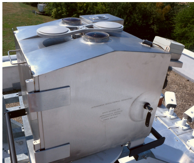
Fig. 1. Digital Autonomous Fireball Observatory (DAFO) with the lens cover open at its site in Ondřejov. The Aurora weather sensor is on the right, next to the GPS receiver. The radiometer window is at the back right corner.
